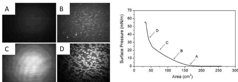
**Figure 3:** Iron oxide nanoparticle isotherm and Brewster angle microscopy images at different surface pressures. With permission from J. Phys. Chem. B 2007, 111(31), 9288-9293. Copyright 2007 American Chemical Society.
