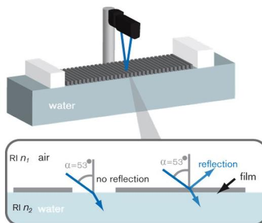
Figure 1: Working principle of Brewster angle microscopy (BAM)
