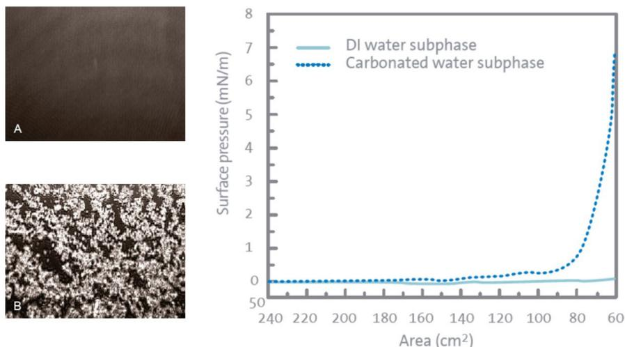
**Figure 2:** (Left) In situ BAM images of A) a freshly prepared graphene oxide - water solution and B) graphene oxide with flotation. (right) The isotherm of graphene oxide with water subphase and carbonated water subphase. With permission from J. Am. Chem. Soc. 2010, 132 (23), pp 8181-8186. Copyright 2010 American chemical society.
