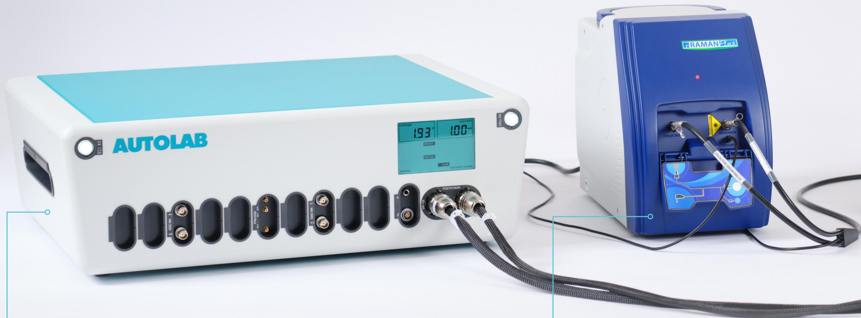
Autolab modular **PGSTAT302N** with an **Electrochemical Impedance Spectroscopy (EIS)** module included.
