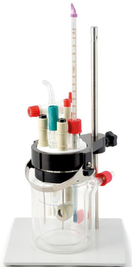
Figure 6 – Overview of the complete setup of the 250 mL corrosion cell
