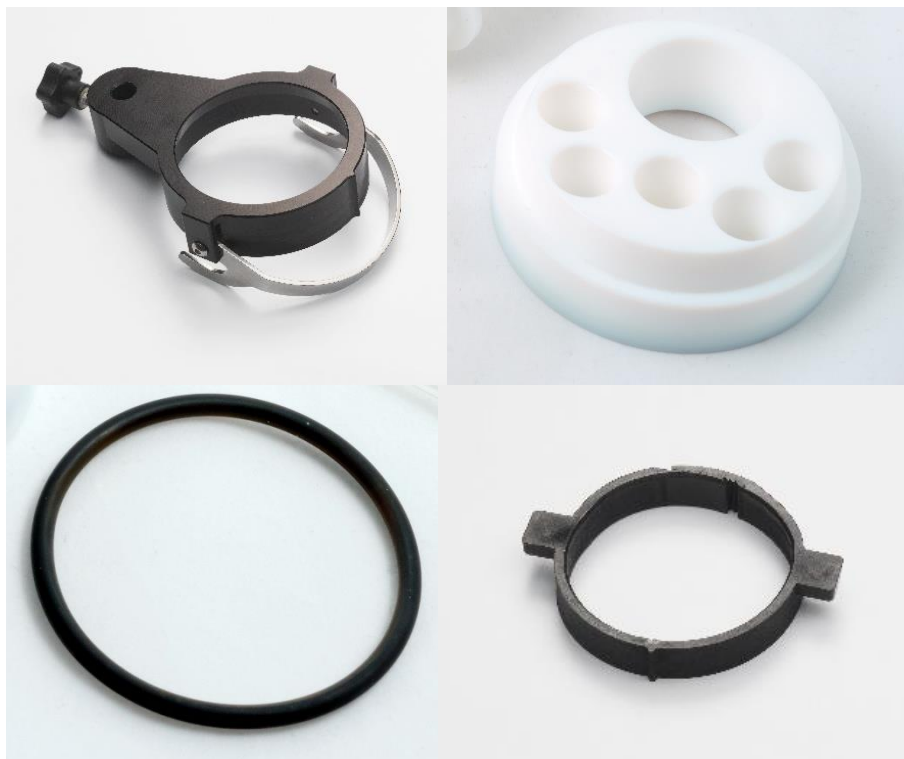
Figure 8 – 250 mL corrosion cell lid consisting of: aluminium clamp, PTFE insert, O-ring and Nylon fixing ring
