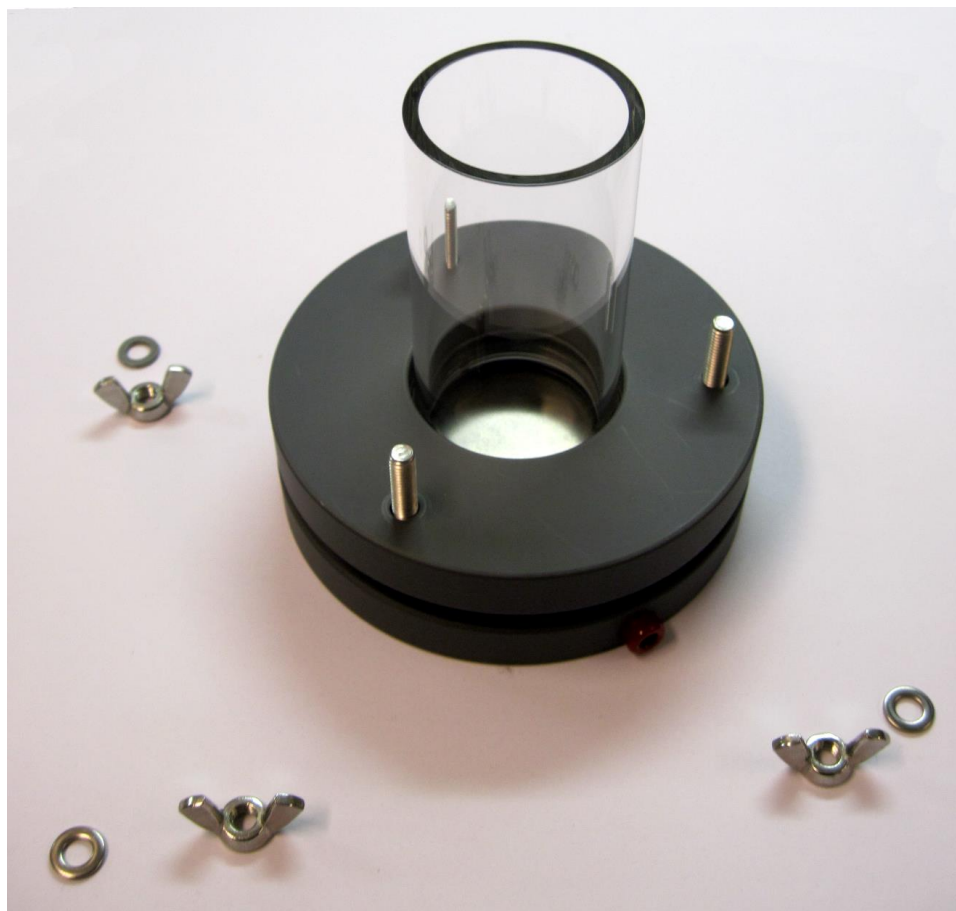
Figure 20 – Close the sample holder by positioning the top part on top of the bottom part of the sample holder
