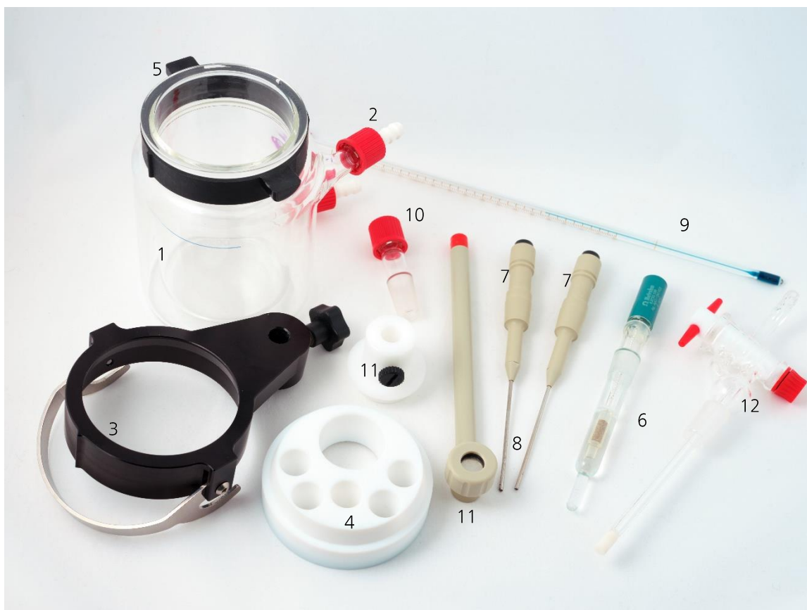
Figure 7 – Individual parts (scope of delivery) of the complete setup of the 250 mL corrosion cell
