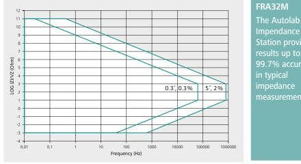
This contour plot is an **accurate** and **precise** representation of the performance of a 302N with FRA32M module in potentiostatic mode.
