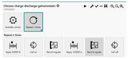
*Figure 710 The default Chrono charge discharge galvanostatic procedure*
