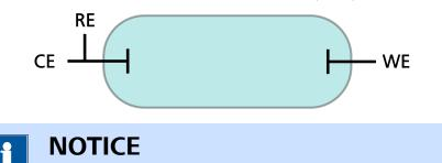
For high current applications it is highly recommended to separately connect the RE and CE to the same electrode. Furthermore, it is recommended to place the RE as close as possible to the electrodes in the cell. This will reduce ohmic losses coming from the connections.
