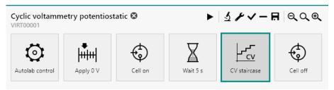
Figure 556 The default Cyclic voltammetry potentiostatic procedure
