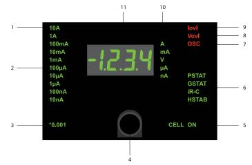
Figure 1120 Overview of the display of the Autolab
