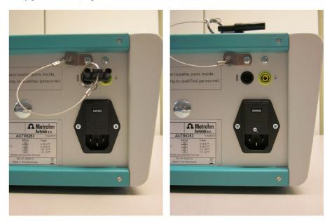
*Figure 1099* The PGSTAT302F can be set to normal mode (left) or to floating mode (right) using the provided short-circuit plug
