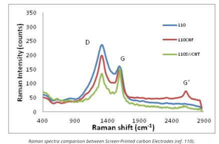
Single-walled carbon nanotubes modified Screen-Printed carbon Electrode (ref. 110SWCNT) and Carbon Nanofibers modified Screen-Printed carbon Electrode (ref. 110CNF), Relationship between D and G bands' intensity provide us information about these materials structure.
