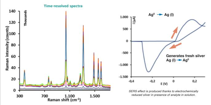
Experimental conditions: Cyclic Voltammogram E0= 0.3V, Evtx1= -0.4V, Evtx2= 0.3V, Step potential= 2 mV,Scan rate= 50 mV/s; Raman's experiment parameters: Integration time 2 s, Laser power= 0.7 V.
