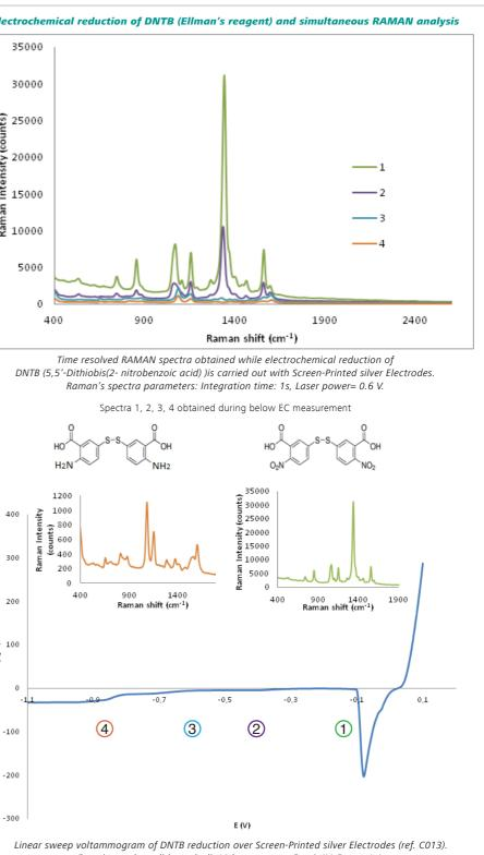
Experimental conditions: Cyclic Voltammogram  $E_0 = 0.1V$ ,  $E_{end} = -1.1$ , Step potential= 5 mV, Scan rate= 25 mV/s;
