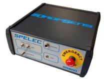
bipotentiostat/galvanostat, and it can be controlled by an excellent spectroelectrochemical software.
