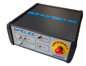
Screen-printed electrodes (refs. DRP-110, DRP-110SWCNT, DRP-110CNT, DRP-110OMC, DRP-110GPH, DRP-110CNF) were placed in a specific cell for this type of devices (DRP-RAMANCELL) coupled with the DRP-RAMANPROBE, which allows to perform the Raman measurements of the electrode surface at optimal focal distance. Integration time was 20 s.
