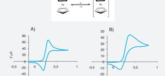
Ferrocene 2 mM in CH<sub>3</sub>CN and LiClO<sub>4</sub> 0.1M. A) Ref. C220AT, Screen-printed gold electrode / lnk AT (Aux.: Au; Ref.: Ag). B) Ref. C550, Screen-printed platinum electrode (Aux.: Pt; Ref.: Ag).
