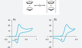
Ferrocene 2 mM in <sup>1</sup>PrOH and LiClO<sub>4</sub> 0.1M. A) Ref. C220AT, Screen-printed gold electrode / Ink AT (Aux.: Au; Ref.: Ag). B) Ref. C550, Screen-printed platinum electrode (Aux.: Pt; Ref.: Ag).
