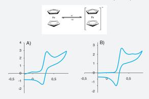
Ferrocene 0,2 mM in DMSO and Bu<sub>4</sub>NPF<sub>6</sub> 0.1M. A) Ref. C220AT, Screen-printed gold electrode / Ink AT (Aux.: Au; Ref.: Ag). B) Ref. C550, Screen-printed platinum electrode (Aux.: Pt; Ref.: Aq).
