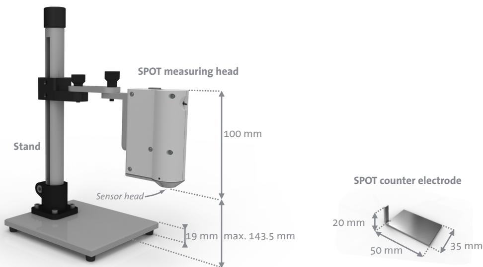
The counter electrode is placed in the subphase with the arm protruding through the subphase surface. This plate is connected to the SPOT measuring head by a cable.
