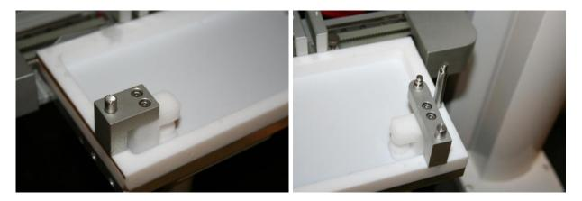
Once the right side ribbon holder is in place add the tightening spring on top of the pole mounted on the right side of the trough.
