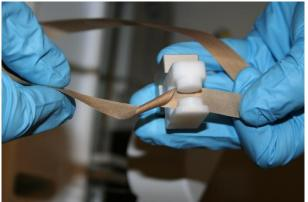
Once the corner holder are in place clean the barriers same way as the holders. After that mount the barriers on the ribbon as shown below. Note that it is easier to mount them when barrier holders are compressed to the center.
