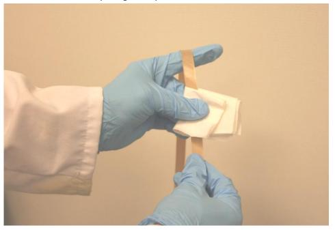
Then mount the ribbon gently on both of the ribbon holders on the trough top. Note that gently twisting the ribbon helps on placing it in the holders. Try to prevent the ribbon from touching any other surface than the clean trough top.
