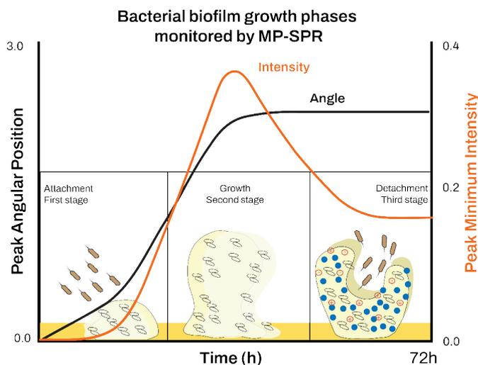
**Figure 2.** *In situ* *Staphylococcus aureus* bacterial biofilm growth phases monitored by MP-SPR (670 nm wavelength). The black and orange lines show the Peak Angular Position (PAP) and Peak Minimum intensity (PMI) changes plotted against time.  $\Delta\text{PMI}$  indicates a stage after bacterial proliferation, which is due to production of extracellular matrix (ECM) and formation of a uniform layer.
