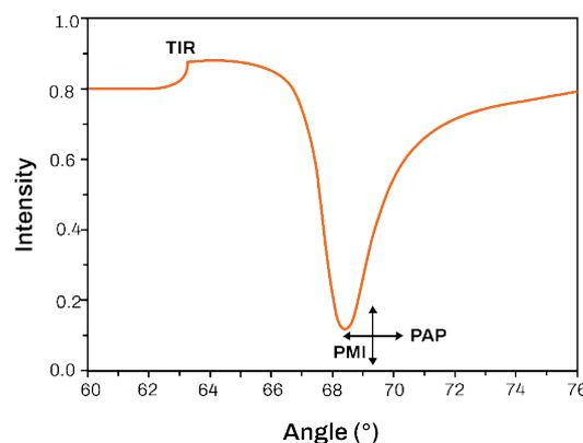
**Figure 1.** MP-SPR instruments measure complete SPR curve continuously, and multiple parameters can be followed in real-time, including Peak Angular Position (PAP), Peak Minimum Intensity (PMI) and Total Internal Reflection (TIR) angle.
