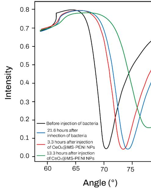
**Figure 4.** The unique, complete SPR curve measurement from MP-SPR allows tracking not only peak angle changes but also intensity parameters, which are crucial for this study. Complete MP-SPR curve (at 5 min) before the injection of bacteria (black),  $t = 21.6$  h after the start of the injection of bacteria (blue), 3.3 h (red, time = 25h in Figure 3) and 13.3 h (green,  $t = 35$  h in Figure 3) after the start of the injection of positively charged PEI coated nanoparticles.
