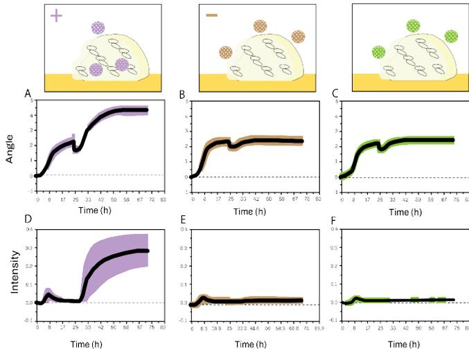
**Figure 3.** Average of real-time MP-SPR responses of the  $\Delta$ PAP (upper graphs) and the  $\Delta$ PMI (lower graphs) during *Staphylococcus aureus* bacterial biofilm growth and interaction of differently charged Nanoparticles (from  $t = 21.6$  hours and onwards).
