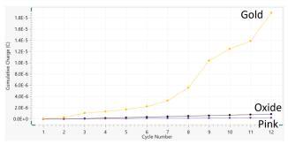
Figure 3 – Cumulative charge vs. cycle number for the three samples
