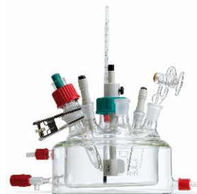
Figure 1 – The Metrohm Autolab 1 L corrosion cell.
