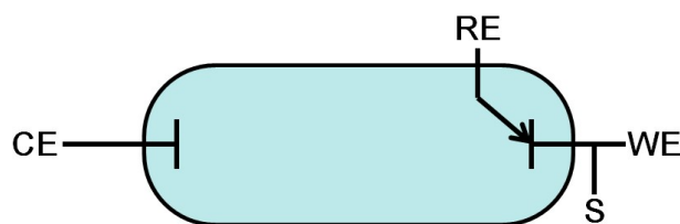
Figure 2 – Schematic overview of the three electrode setup
