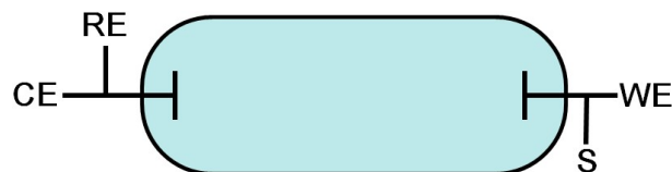
Figure 1 – Schematic overview of the two electrode setup
