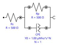
the effective capacitance  $C_{eff}$  can be calculated with the following Equation:
