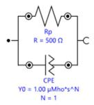
the effective capacitance can be calculated with the following Equation:
