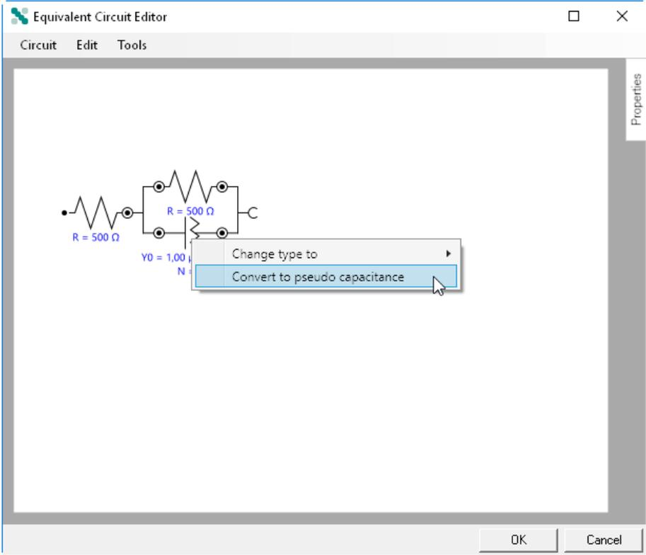
Figure 489 Converting a Q element to a pseudo capacitance
