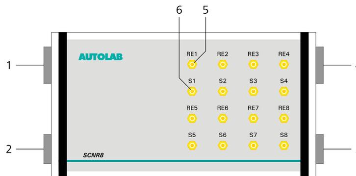
Figure 1235 The connections provided by the MUX-SCNR8 switch box
