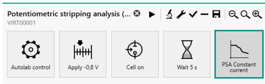
Figure 699 The default Potentiometric stripping analysis (Constant current) procedure
