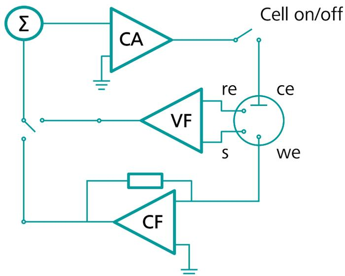
Figure 1059 Schematic representation of the analog circuits of the Autolab in a four electrode system
