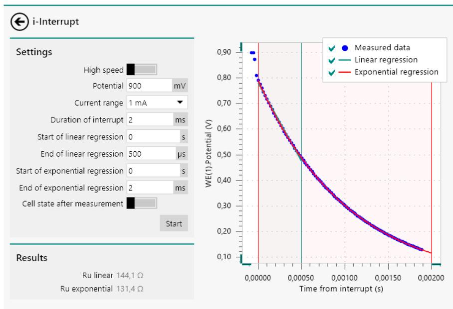
Figure 29 The current interrupt tool now provides the possibility to set the cell end state
