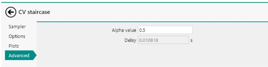
Figure 764 The Delay value is automatically updated when the Alpha value is modified
