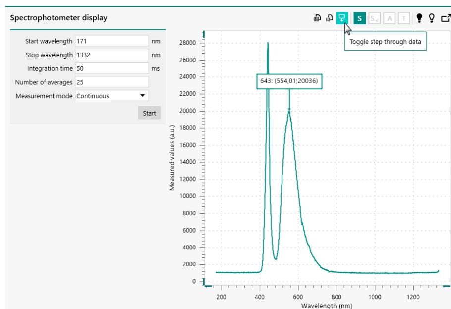
*Figure 25* The *Step through data* option can be used in the Spectrophotometer control panel
