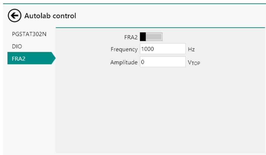
Figure 1206 The FRA2 module settings defined in the Autolab control command
