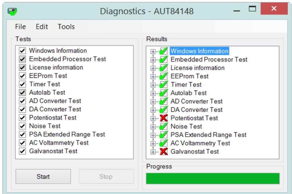
Figure 1258 A failed test will be indicated in the diagnostics tool
