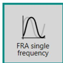
This command can be used to perform an impedance spectroscopy measurement at a single frequency. This command requires the optional **FRA32M** or **FRA2** module.
