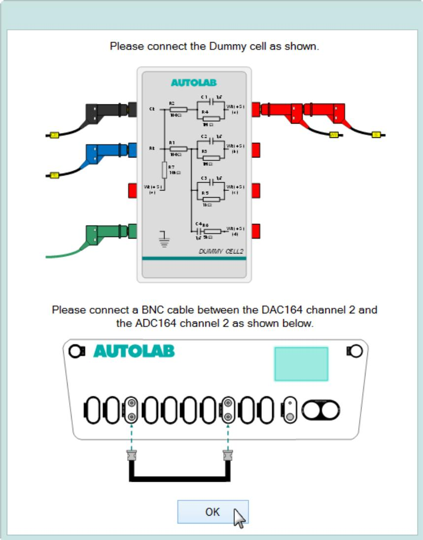
Figure 1256 A visual reminder is shown at the beginning of the Diagnostics test
