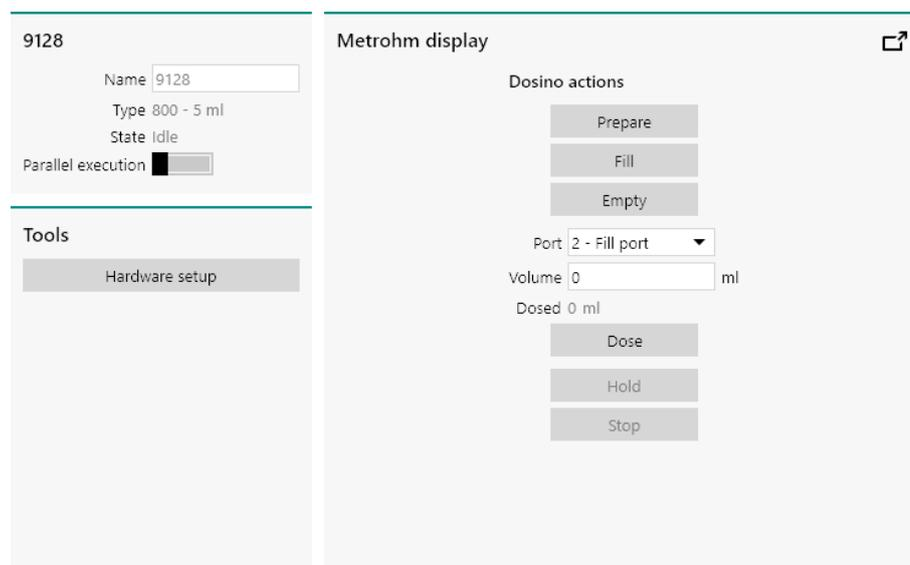
Figure 159 The Metrohm Dosino control panel
