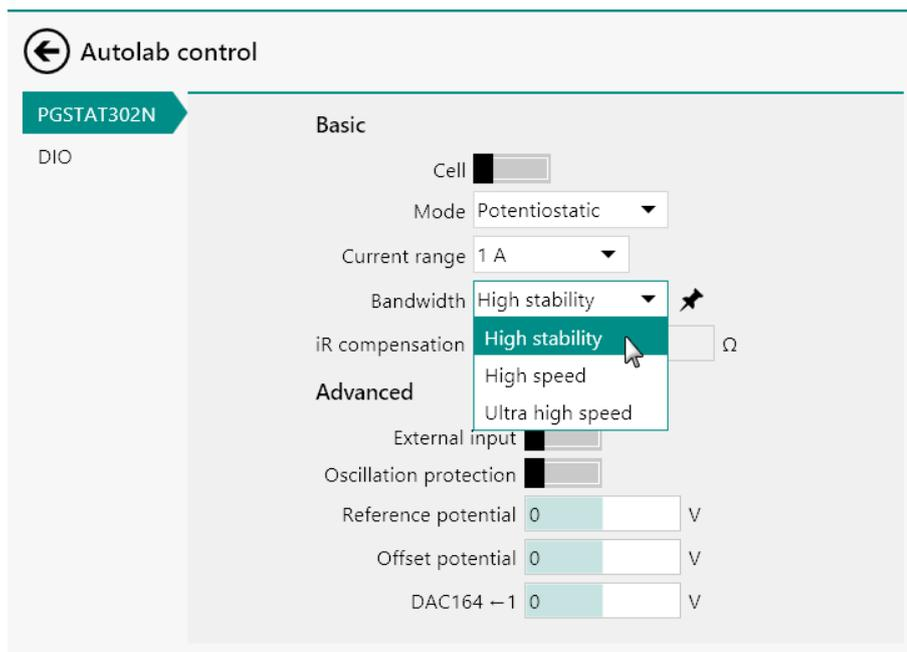
Figure 1062 The instrument bandwidth is defined in the Autolab control command
