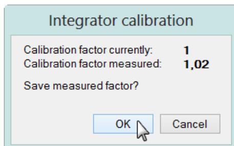
Figure 1259 The value of the measured Integrator calibration factor is displayed at the end of the integrator test
