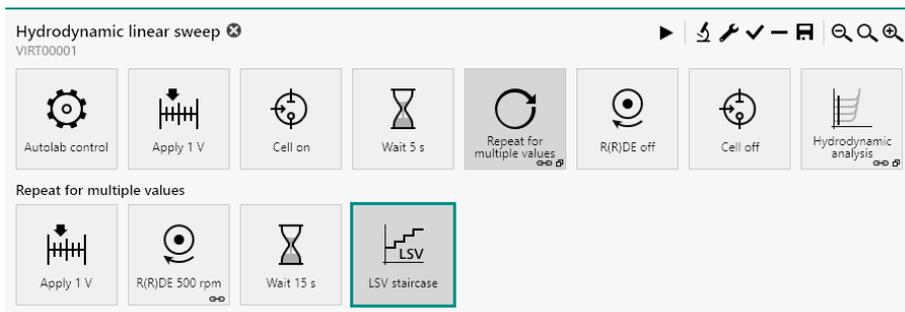
Figure 776 The Hydrodynamic linear sweep voltammetry procedure
