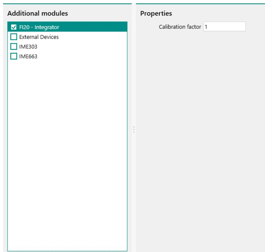
*Figure 1197* The on-board integrator is automatically selected for applicable instruments
