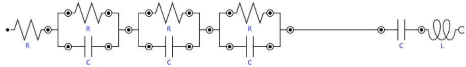
*Figure 502* Circuit used in for Kramers-Kronig test on impedance presentation
