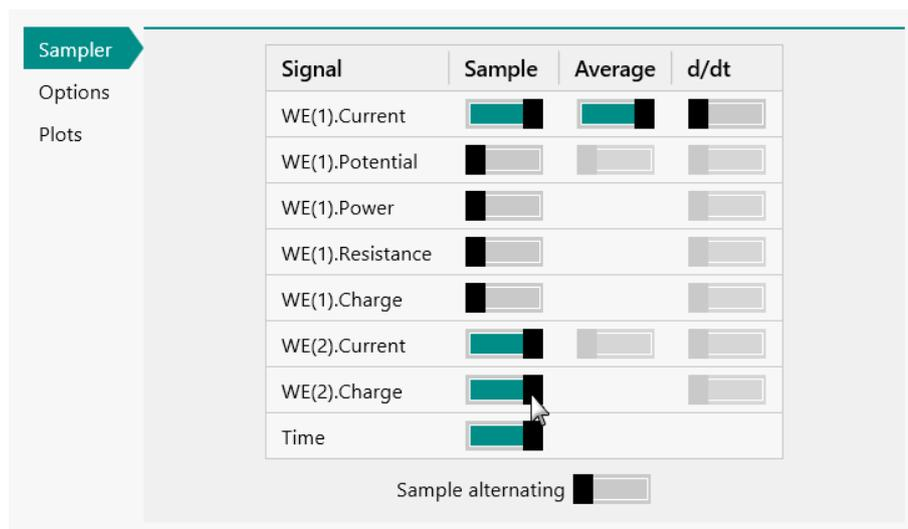
Figure 1144 The BA module provides the WE(2).Charge and WE(2).Current signals
