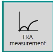
This command can be used to perform an impedance spectroscopy measurement through a frequency scan. This command requires the optional **FRA32M** or **FRA2** module.
