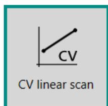
This command can be used to perform a linear scan cyclic voltammetry measurement, in potentiostatic. This method can only be used with instrument fitted with the optional **SCAN250** or **SCANGEN** module.
