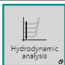
This command can be used to perform a Levich and Koutecký-Levich analysis on hydrodynamic data.
