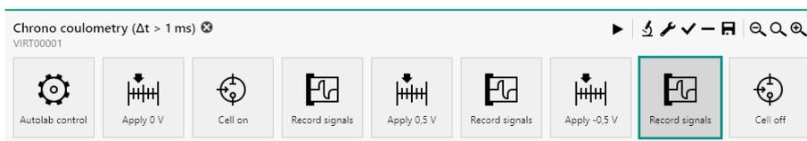
Figure 658 The default Chrono coulometry ( $\Delta t > 1$  ms) procedure
