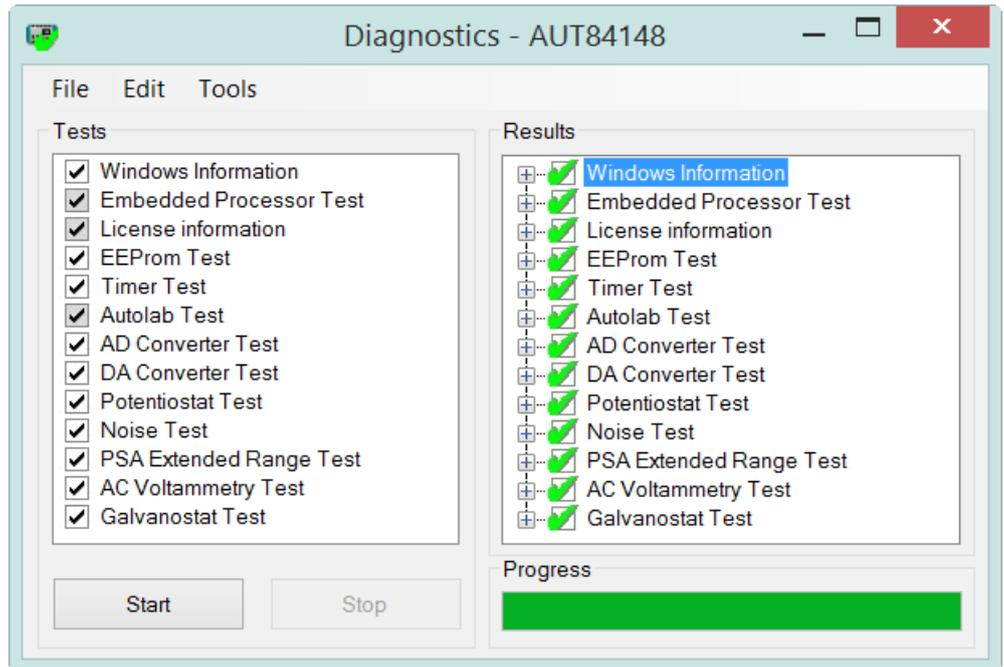
Figure 1257 The diagnostics report after all the tests have been performed successfully
