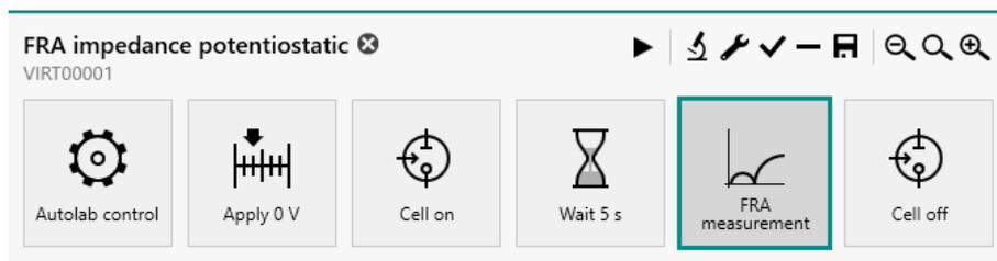
Figure 702 The default FRA impedance potentiostatic procedure
