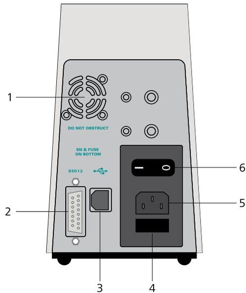
Figure 1084 The back plane of the PGSTAT101
