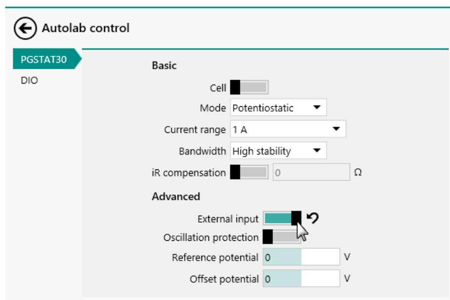
Figure 1102 The **Ein** connection is enable or disabled in the Autolab control command
