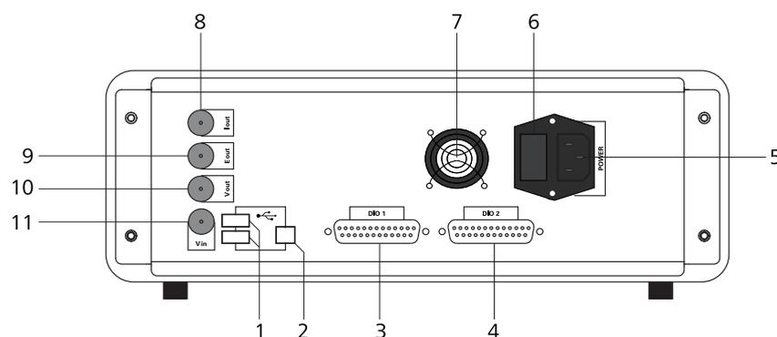
*Figure 1106 Overview of the back plane of the  $\mu$ Autolab type III*
