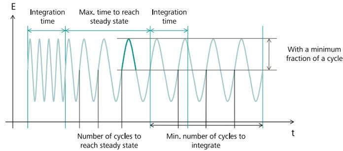
Figure 348 Overview of the timing properties (Integration time: 2 s, Minimum integration cycles: 4, Number of cycles to wait for steady state: 4, Maximum time to reach steady state: 4 s, Minimal cycle fraction of to wait for steady state: 0.5)
