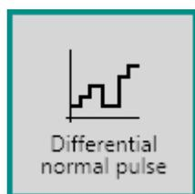
This command can be used to perform a differential normal pulse voltammetry measurement, in potentiostatic conditions.
