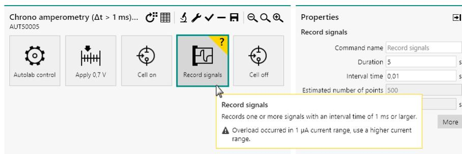
Figure 1068 A warning is displayed if the linearity limit is exceeded during a measurement
