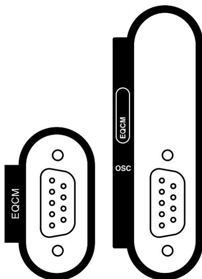
Figure 1193 The front panel labels of the EQCM module (left: EQCM module in PGSTAT, right: EQCM module in Multi Autolab)
