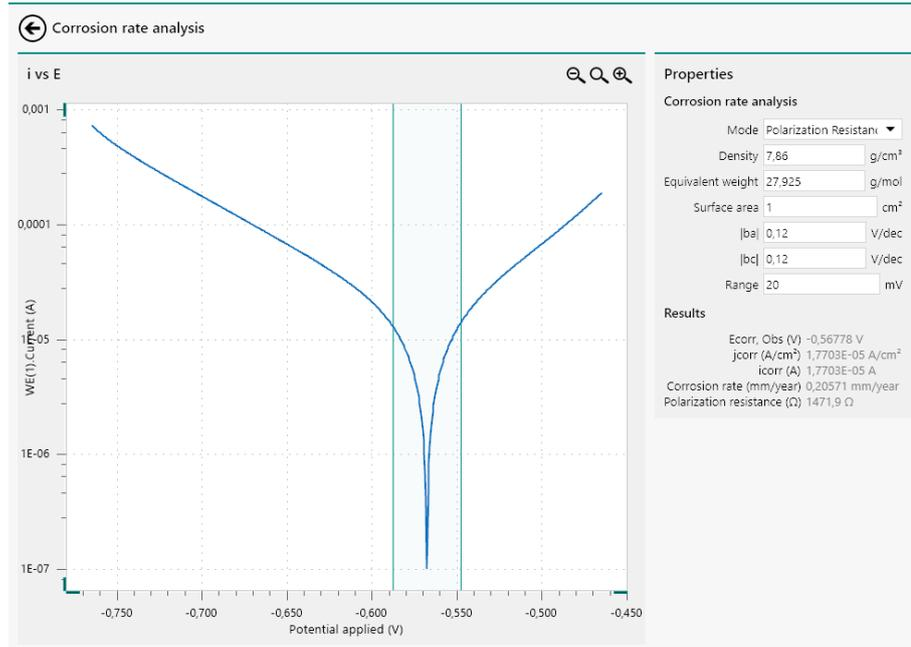
Figure 964 The Polarization Resistance analysis is carried in out in the highlighted range
