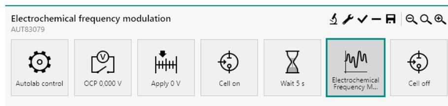
Figure 735 The default Electrochemical Frequency Modulation procedure
