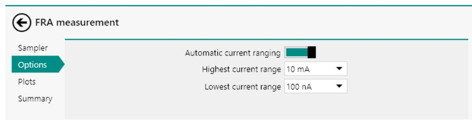
Figure 728 The options of the FRA measurement command
