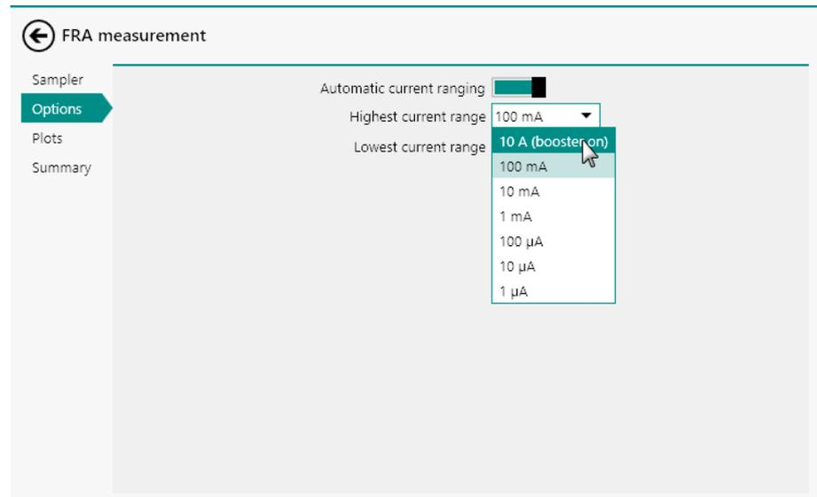
Figure 350 The current range of the Booster10A and Booster20A is available in the Automatic current ranging option
