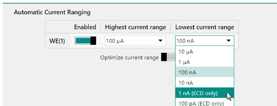
Figure 1171 The ECD current ranges are available in the Automatic current ranging option
