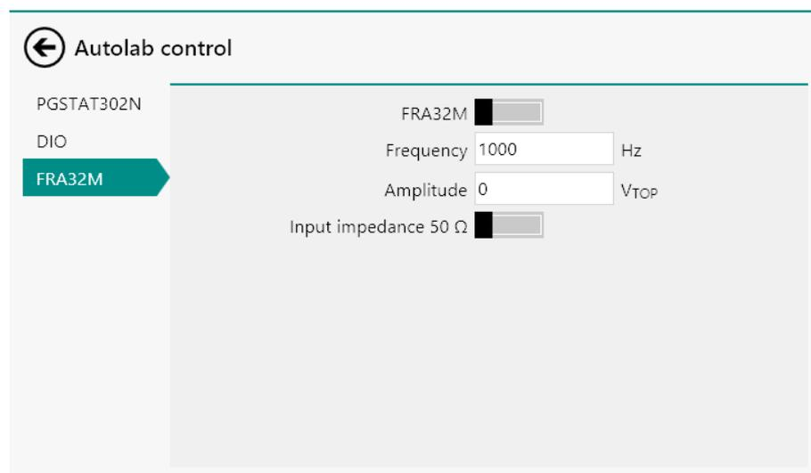
Figure 1212 The FRA32M module settings defined in the Autolab control command
