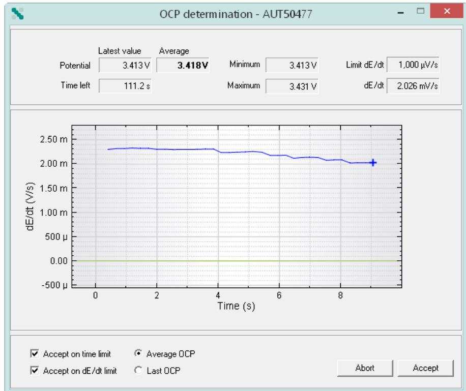
Figure 293 The OCP determination window displayed when the OCP command is executed
