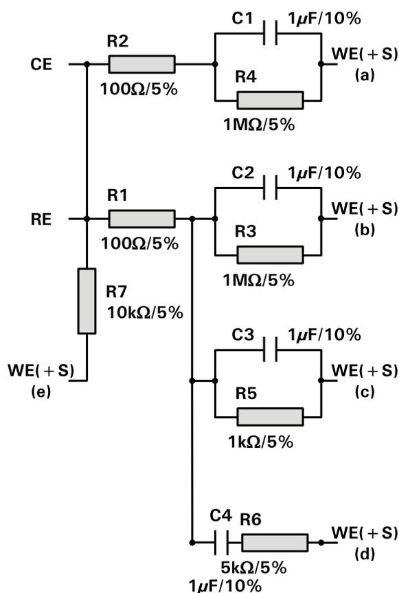
Figure 1127 Component values and tolerances used in the Autolab dummy cell 2
