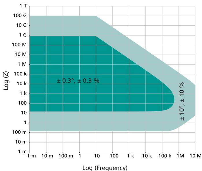
Figure 1179 Contour map of the ECI10M/PGSTAT302N/FRA32M combination
