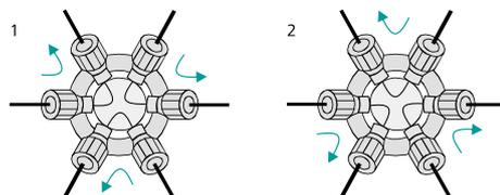
Figure 520 The positions of the injection valve
