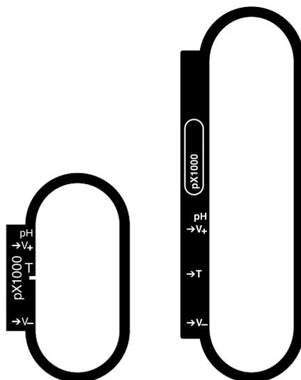
Figure 1246 The front panel labels of the pX1000 module (left: pX1000 module in PGSTAT, right: pX1000 module in Multi Autolab)
