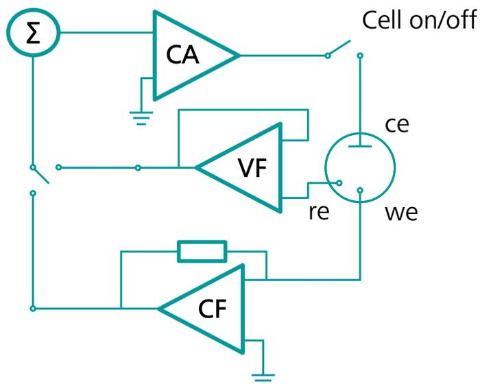
Figure 1060 Schematic representation of the analog circuits of the Autolab in a three electrode system
