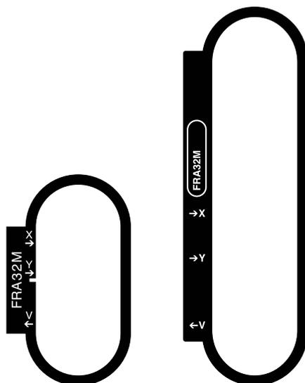
Figure 1215 The front panel labels of the FRA32M module (left: FRA32M module in PGSTAT, right: FRA32M module in Multi Autolab)
