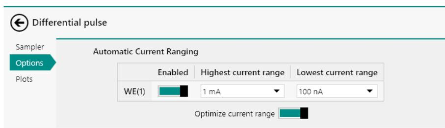
Figure 630 The options of the Differential pulse command
