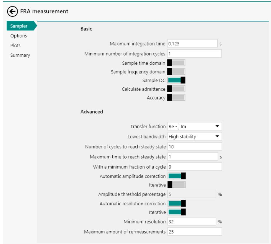
Figure 704 The sampler of the FRA measurement command
