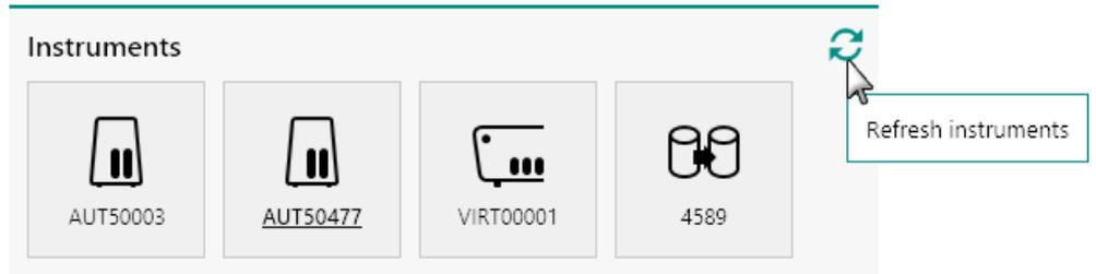
Figure 78 Clicking the refresh button will update the content of the Instruments panel
