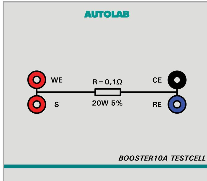
Figure 1133 The BOOSTER10A test cell
