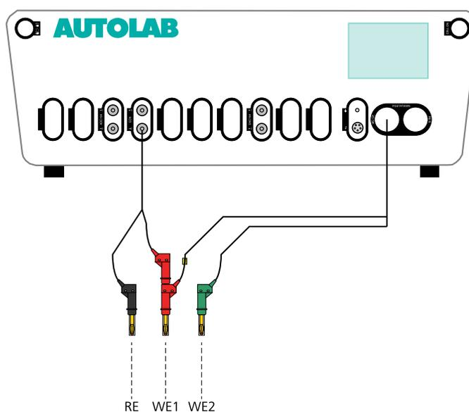
Figure 1188 Overview of the electrode connections for ECN measurements
