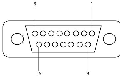
Figure 1123 The DIO12 connector layout
