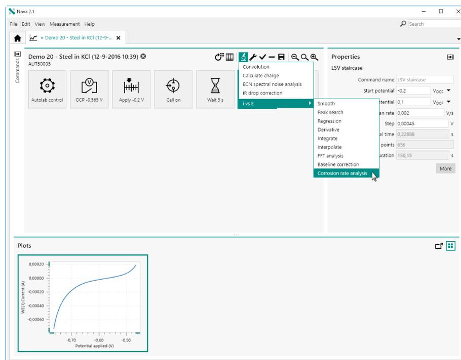
Figure 956 Adding a Corrosion rate analysis command to the linear polarization data
