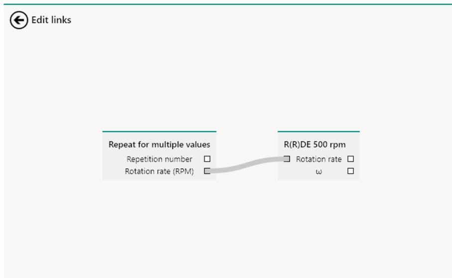
Figure 595 The link used to control the rotation rate of the R(R)DE
