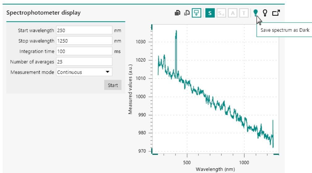
Figure 149 Saving a measured spectrum as Dark spectrum
