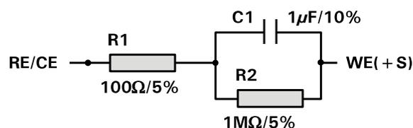
Figure 1130 Component values and tolerances used in the internal dummy cell
