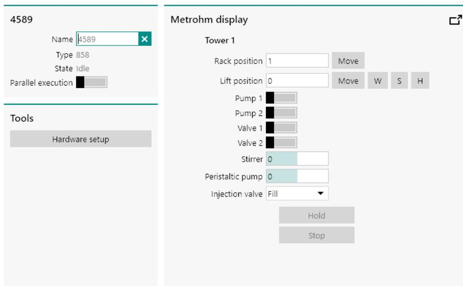
Figure 167 The Metrohm Sample Processor control panel
