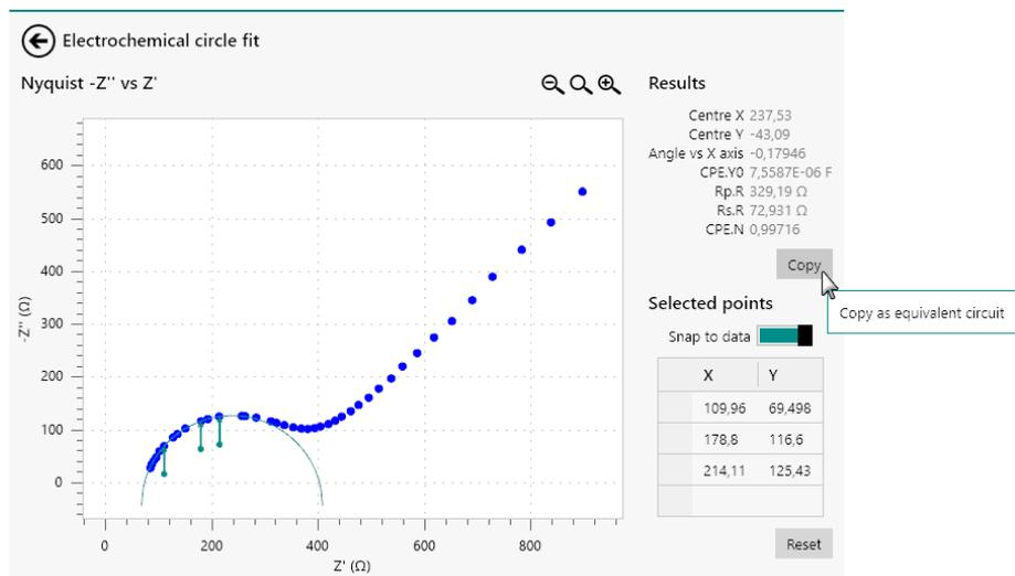
Figure 976 Copy the results as an equivalent circuit
