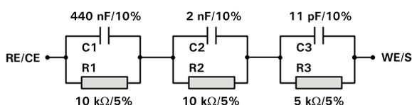
Figure 1132 Component values and tolerances used in the ECI10M test cell
