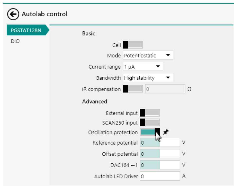
Figure 1066 The oscillation protection can be enabled or disabled in the Autolab control command
