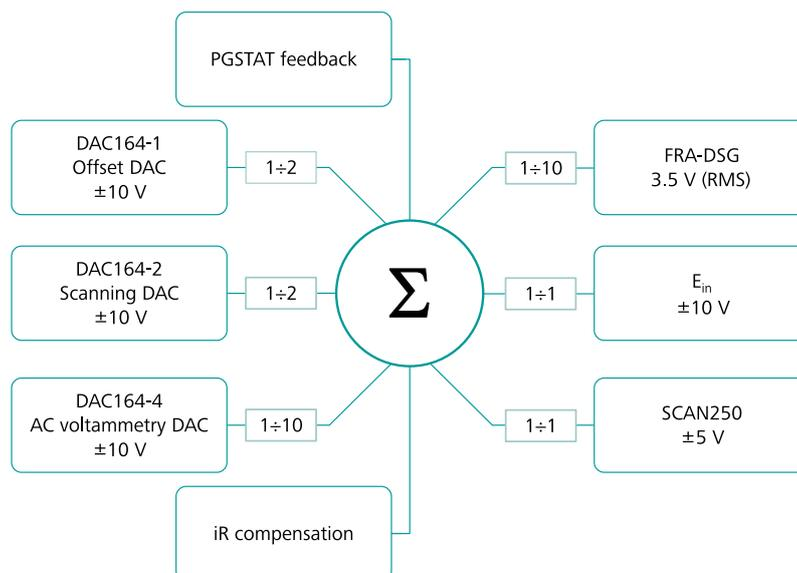
Figure 1061 Schematic representation of the summation point of the Autolab
