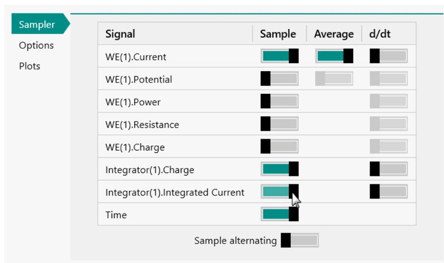
Figure 1195 The FI20 module and on-board integrator provide the Integrator(1).Charge and Integrator(1).Integrated Current signals
