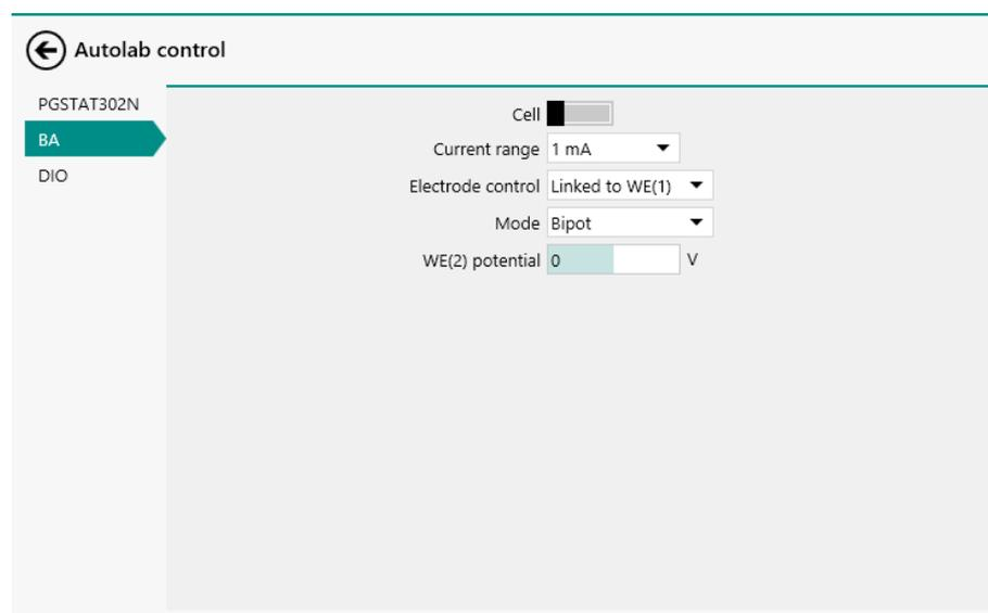
Figure 1146 The BA module settings are defined in the Autolab control command
