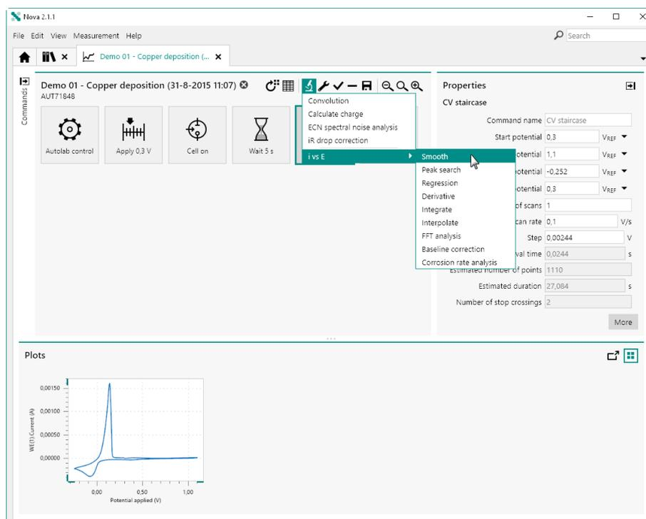
Figure 15 Adding a Smooth command to the *i vs E* plot
