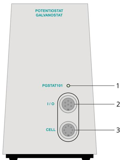
Figure 1082 The front panel of the PGSTAT101
