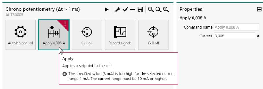
Figure 1067 An error is displayed when the applied current exceeds the linearity limit of the active current range
