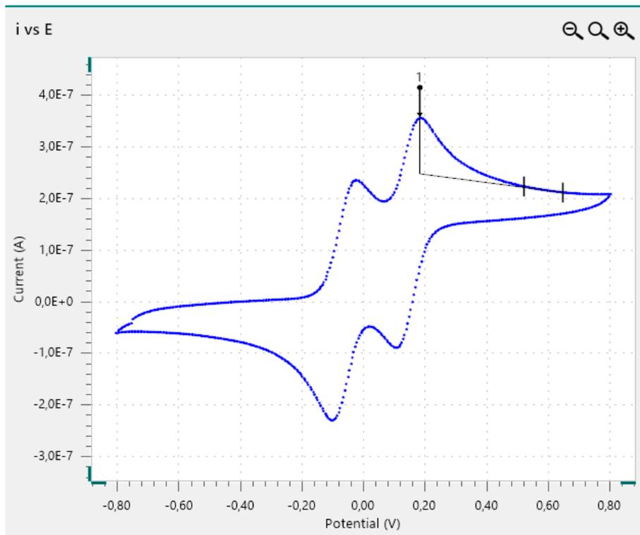
Figure 913 Manual peak search using the linear rear tangent baseline
