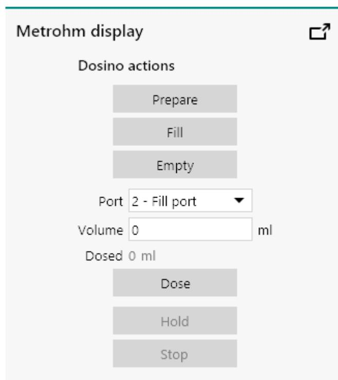
Figure 164 The manual controls of the Dosino
