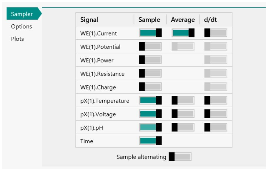
Figure 1243 The pX1000 module provides the pX1000(1).Temperature, pX1000(1).Voltage and pX1000(1).pH signals
