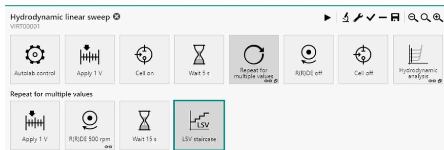
Figure 808 The default Hydrodynamic linear sweep procedure
