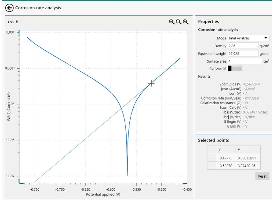
Figure 959 Defining the points for the anodic Tafel slope
