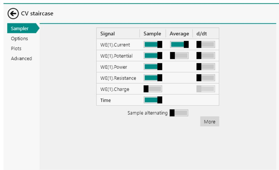
Figure 739 The sampler defines which signals are measured or calculated by the command
