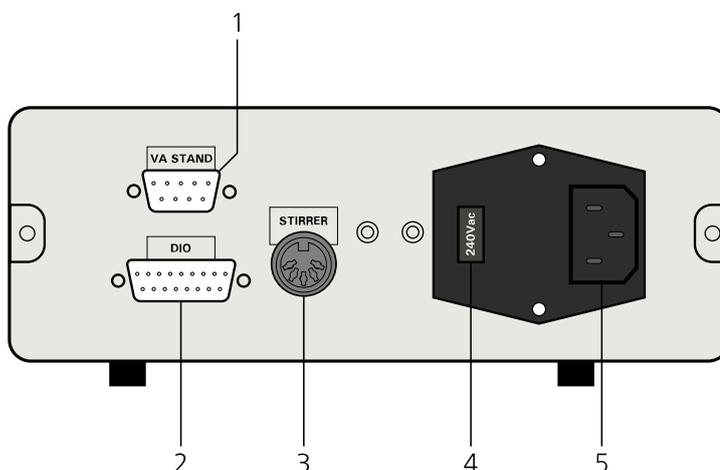
Figure 1225 Overview of the back plane of the IME663
