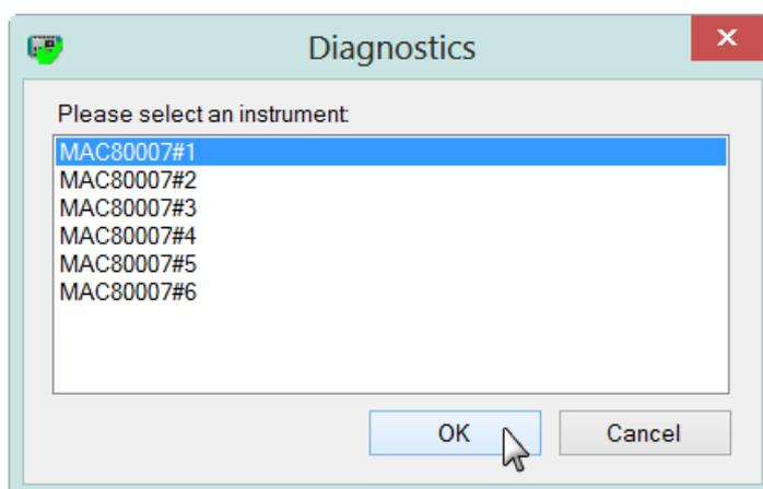
Figure 1255 A selection menu identifying the M101 or M204 modules by position is displayed when a Multi Autolab is detected by the diagnostics application
