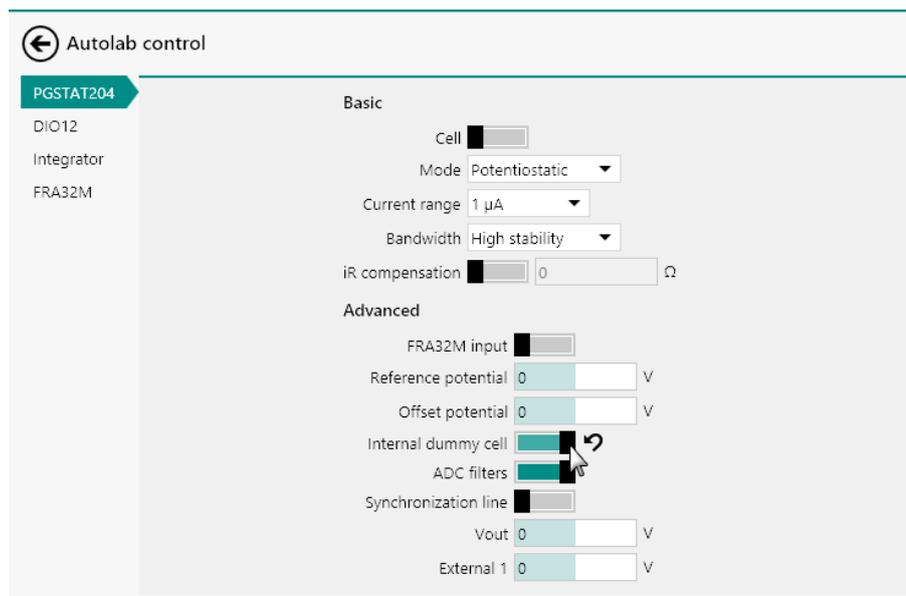
Figure 1129 The internal dummy cell can be activated using the dedicated toggle in the Autolab control command
