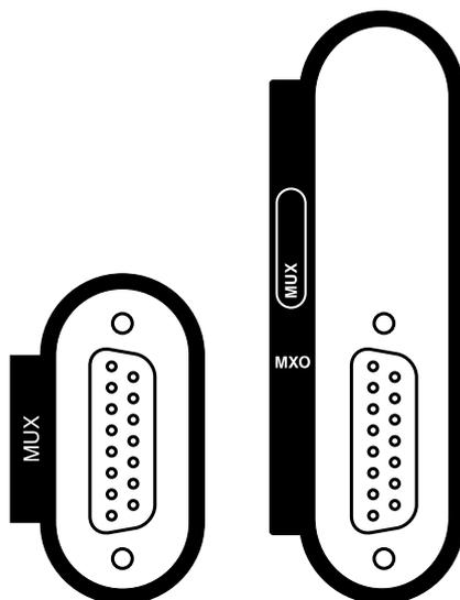
Figure 1233 The front panel labels of the MUX module (left: MUX module in PGSTAT, right: MUX module in Multi Autolab)
