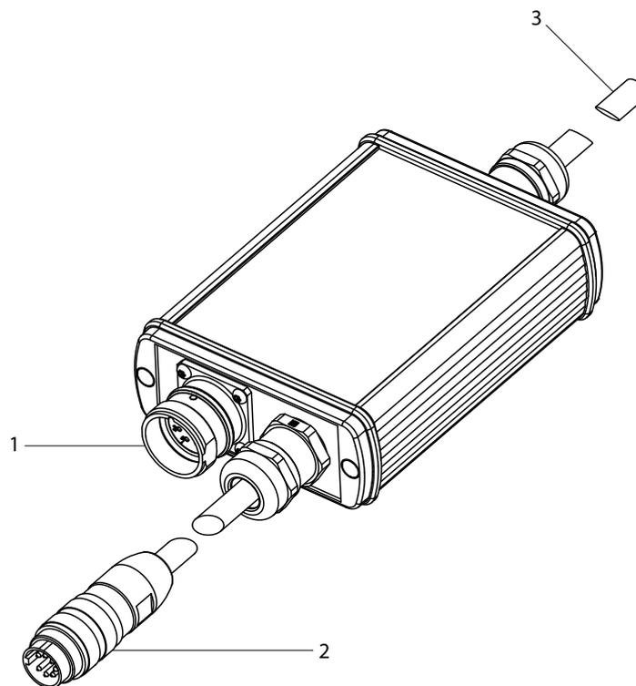
Figure 1159 The cell adapter cable assembly
