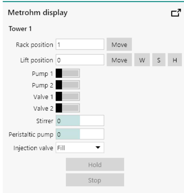
Figure 172 The manual controls of the Sample Processor
