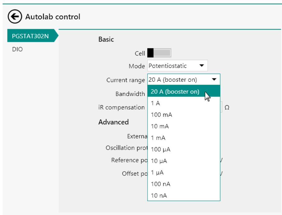
Figure 1162 The Booster20A is controlled by the current range
