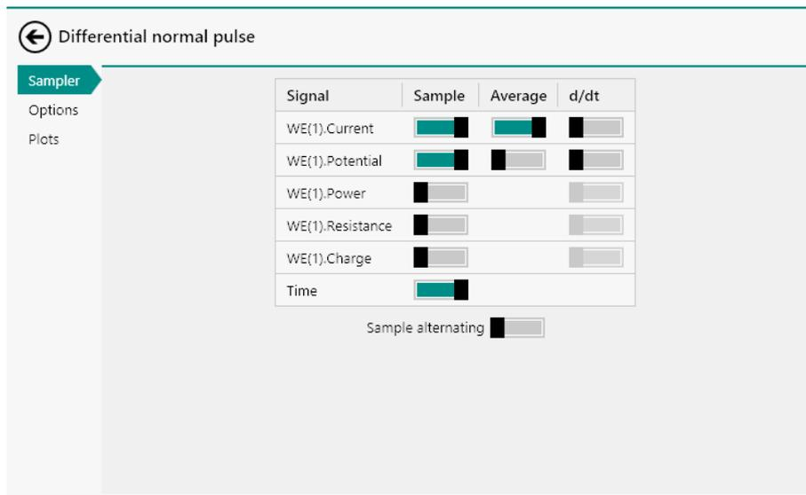
Figure 636 The sampler of the Differential normal pulse command
