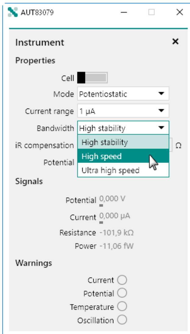
Figure 1063 The instrument bandwidth can be specified directly from the Autolab display panel
