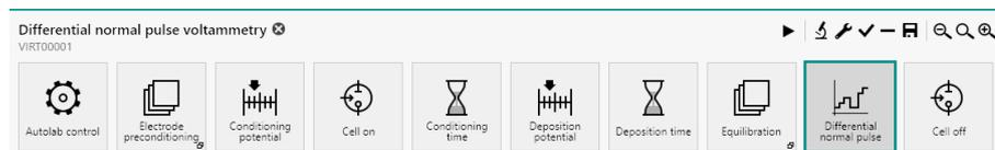
Figure 632 The default Differential normal pulse voltammetry procedure
