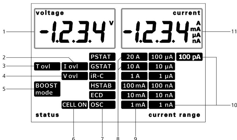
Figure 1070 Overview of the display of the Autolab
