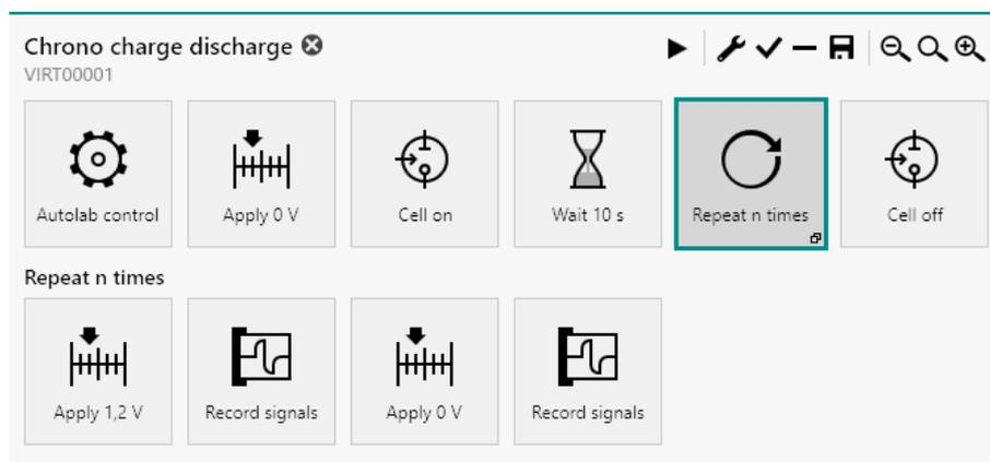
Figure 691 The default Chrono charge discharge procedure
