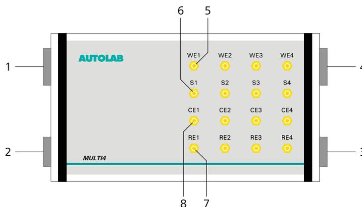
Figure 1234 The connections provided by the MUX-MULTI4 switch box
