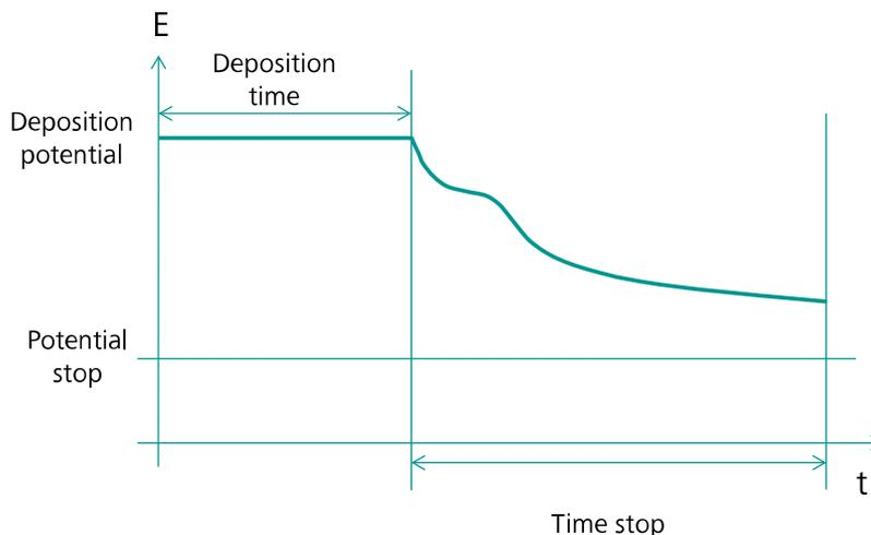
*Figure 321* A typical potentiometric stripping analysis measurement
