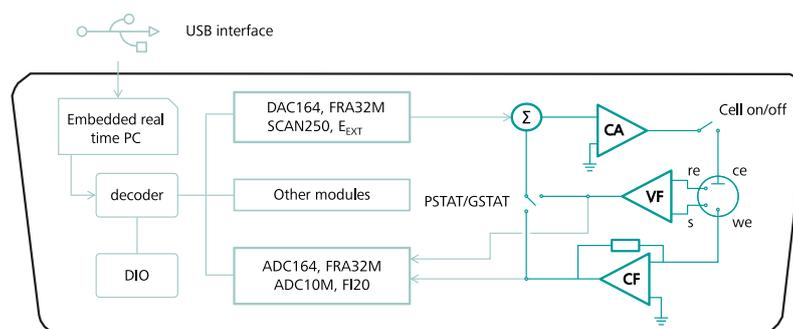
Figure 1058 Schematic representation of the Autolab potentiostat/galvanostat
