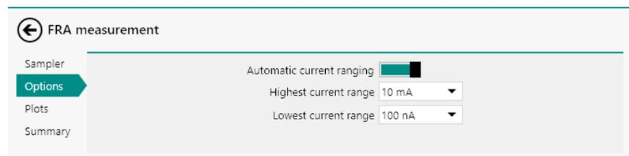
Figure 705 The options of the FRA measurement command
