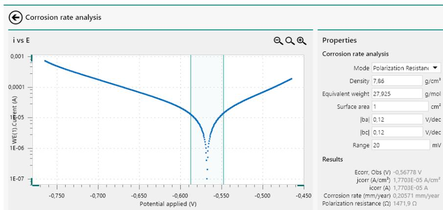
Figure 38 The Linear polarization method has been added to the Corrosion rate analysis command
