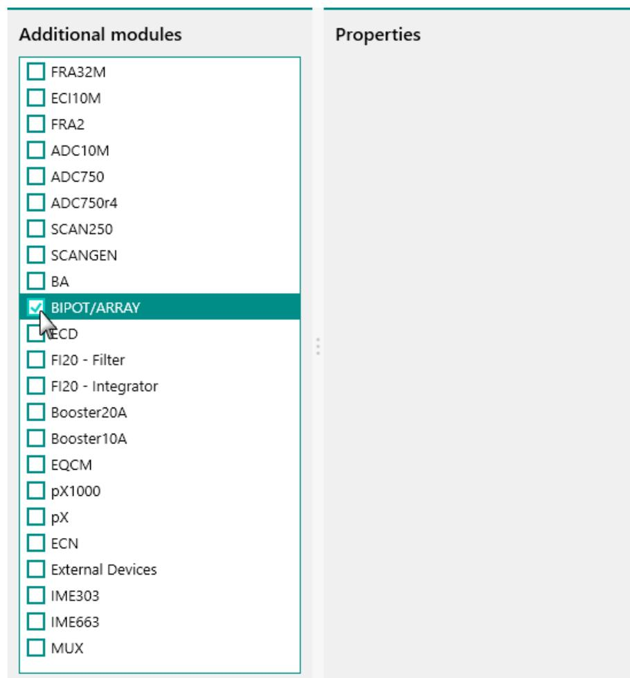
Figure 1150 The BIPOT/ARRAY module is selected in the hardware setup
