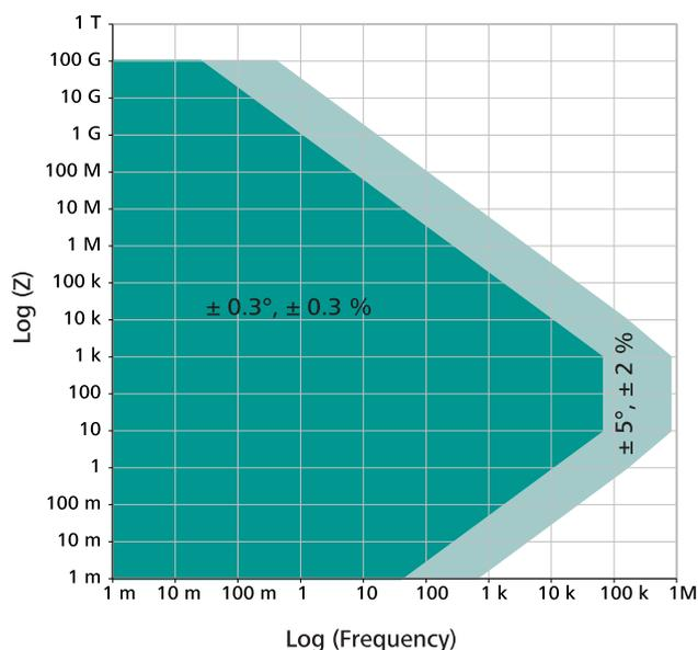
*Figure 1208* Contour map of the PGSTAT302N/FRA2 combination
