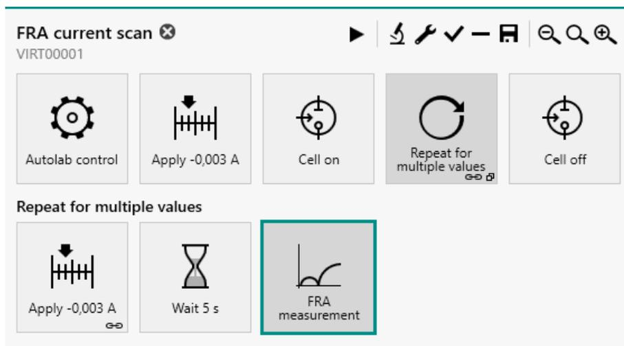
Figure 718 The default FRA current scan procedure
