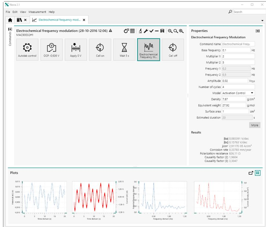
Figure 37 Example of an EFM measurement
