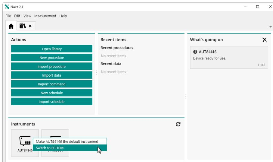
Figure 59 The electrochemical interface can be directly selected through the Dashboard
