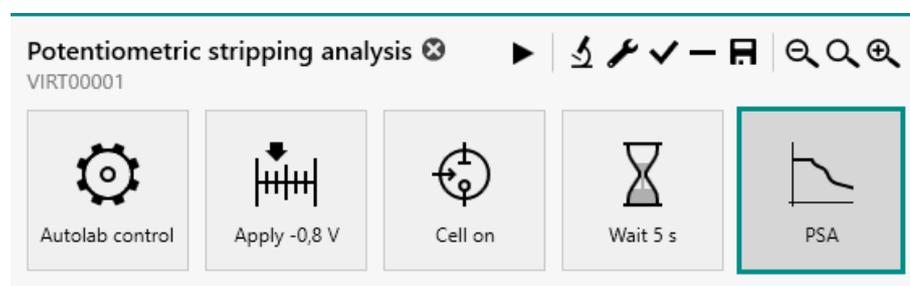
Figure 696 The default Potentiometric stripping analysis procedure
