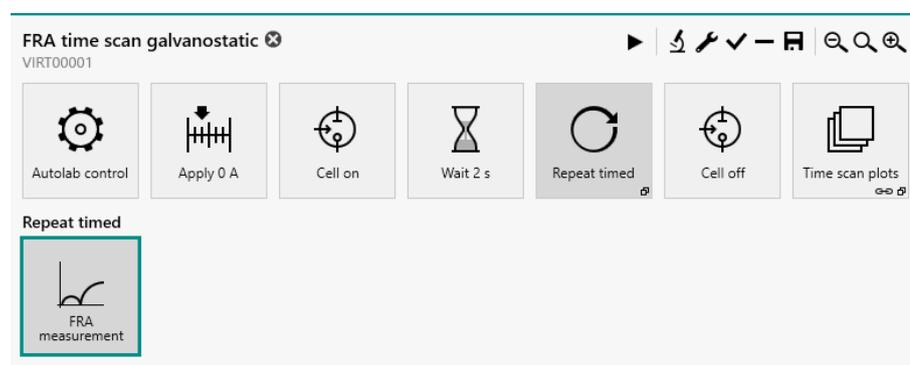
Figure 730 The default FRA time scan galvanostatic procedure
