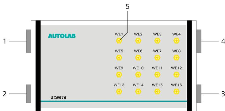
Figure 1236 The connections provided by the MUX-SCNR16 switch box
