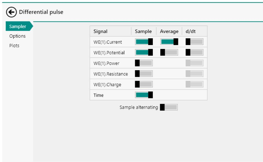
Figure 629 The sampler of the Differential pulse command
