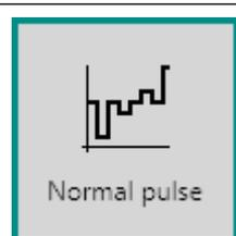
This command can be used to perform a normal pulse voltammetry measurement, in potentiostatic conditions.
