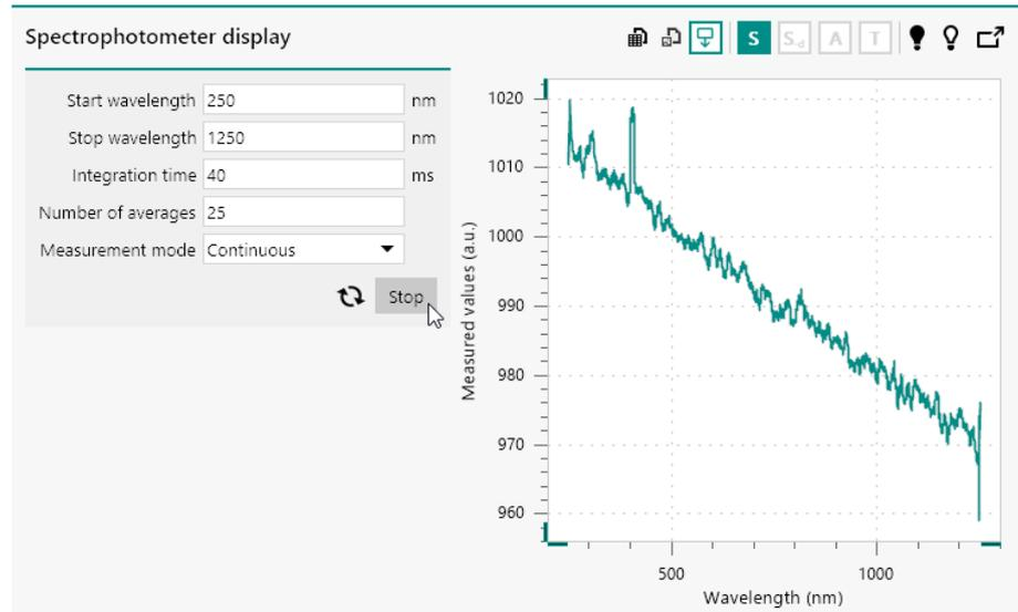
Figure 147 Measured spectra are displayed in the plot on the right-hand side
