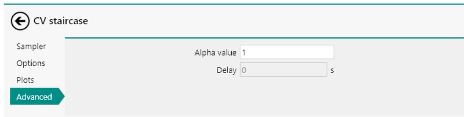
Figure 761 The *Alpha value* property is available for the CV staircase and LSV staircase command
