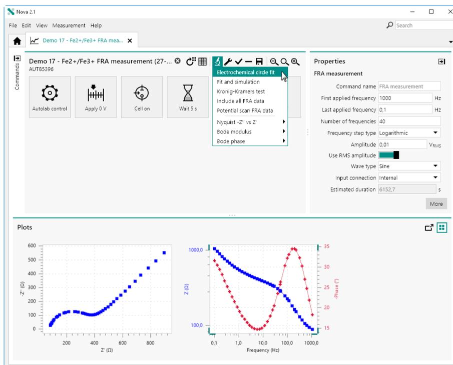
Figure 966 Adding a Electrochemical circle fit command to impedance data
