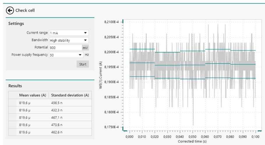
Figure 28 The Check cell tool can now be used to check the noise level
