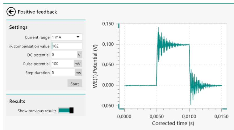
Figure 101 Oscillation is detected when the  $R_u$  value is overcompensated
