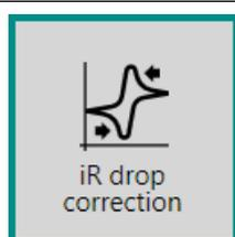
This command can be used to correct measured data for ohmic drop losses.
