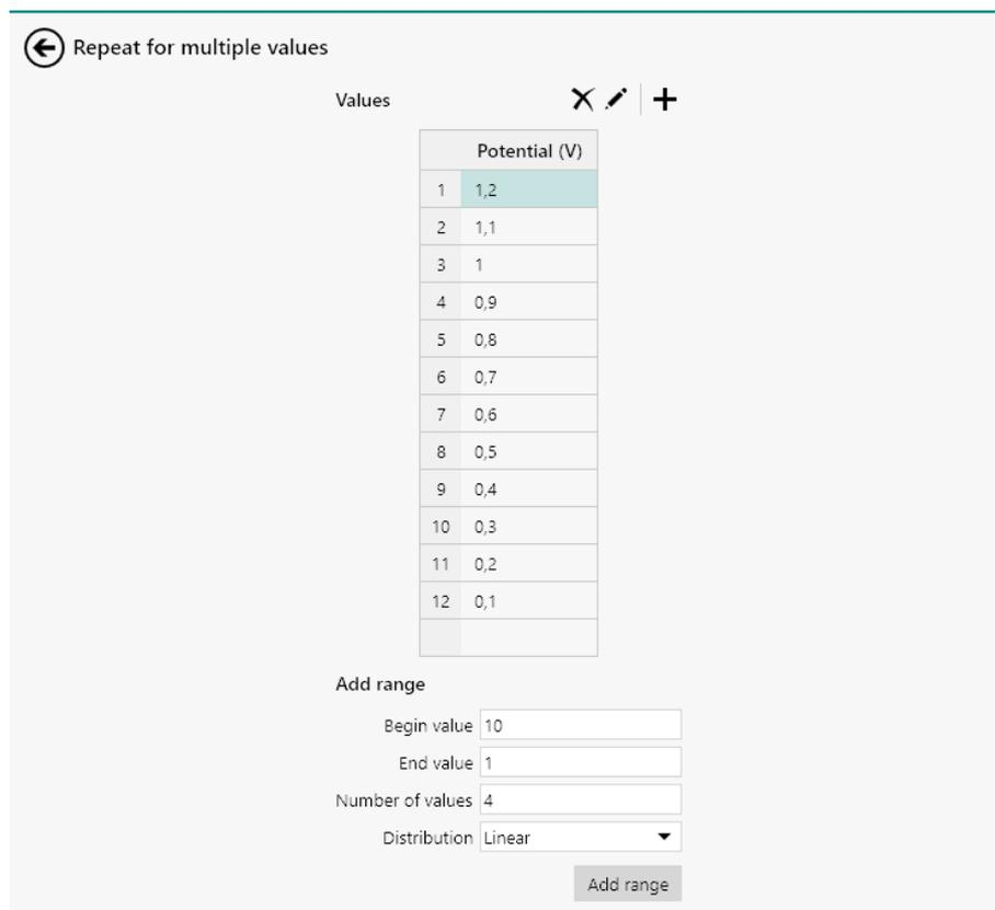
Figure 712 The repeat loop using the default FRA potential scan procedure
