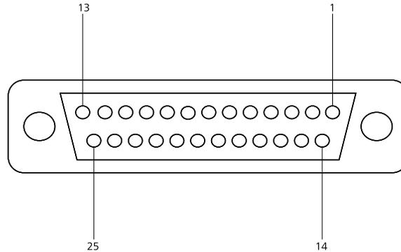
*Figure 1122* The DIO48 connector layout
