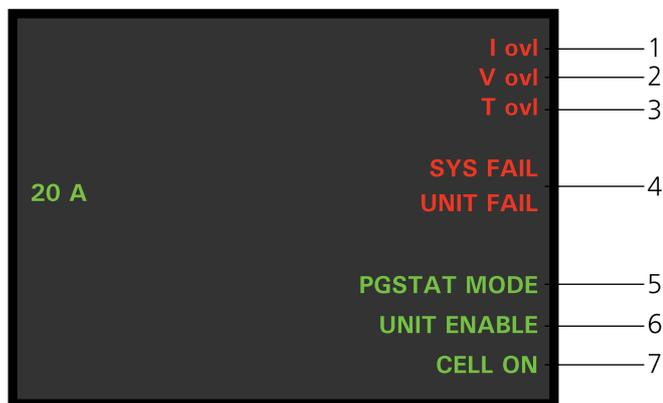
Figure 1164 Overview of the display of the Booster20A
