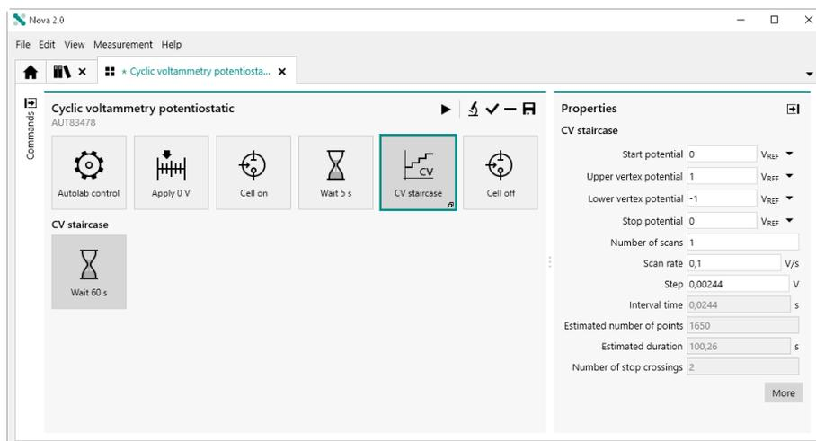
Figure 64 When commands are stacked, the Estimated duration takes underlying commands into account
