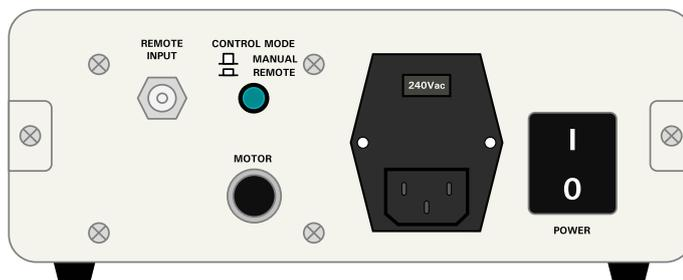
Figure 587 The back plane of the Autolab motor controller
