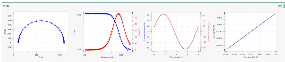
Figure 1216 The data measured by the TestFRA procedure
