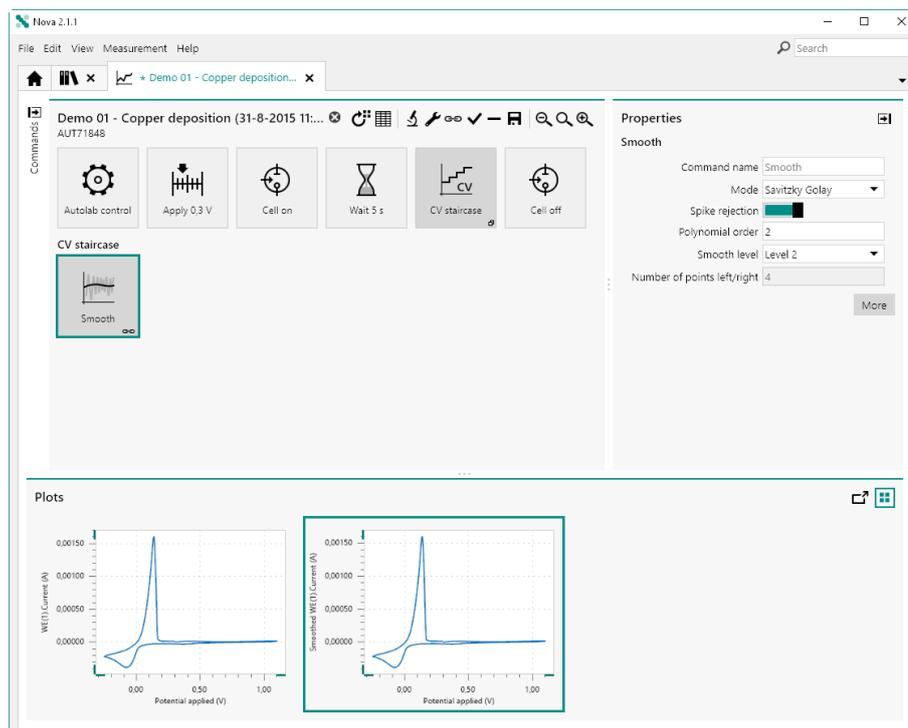
Figure 16 Smoothed WE(1). Current vs Potential applied plot is created
