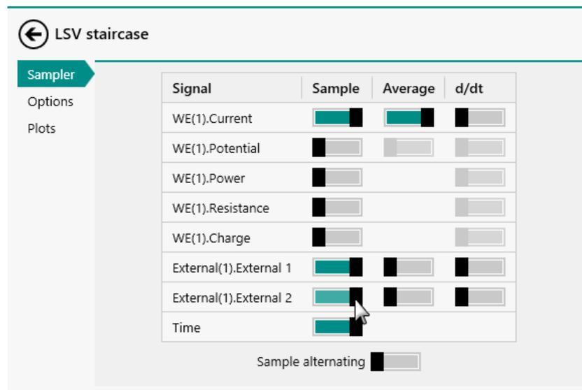
Figure 1109 The ADC164 module provides the External(1).External 1 and External(1).External 2 signals
