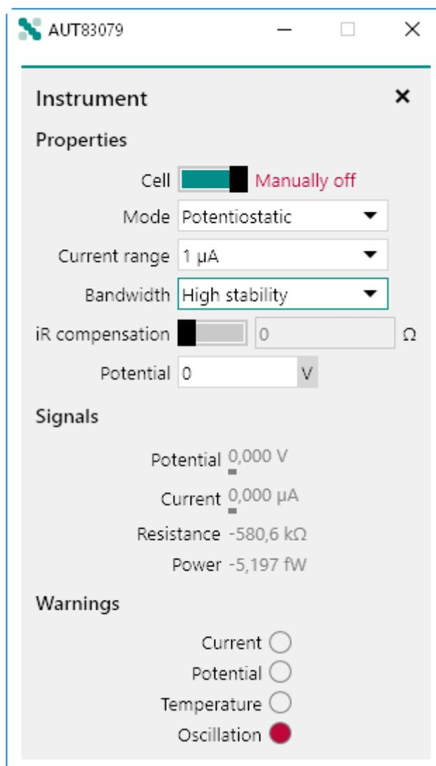
Figure 1065 The oscillation status is reported in the Autolab display panel
