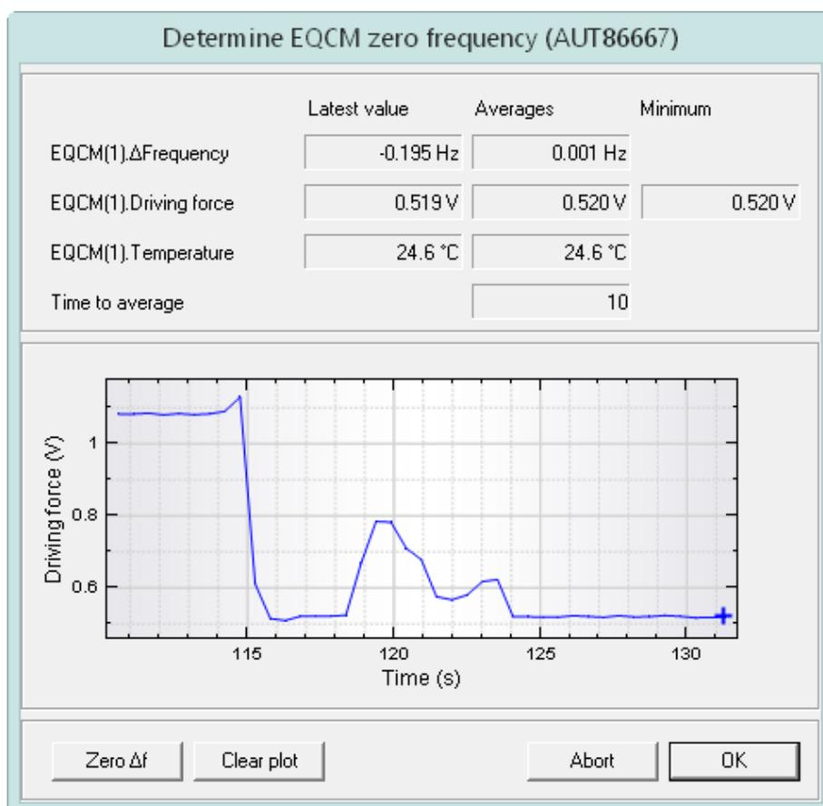
Figure 296 The Determine EQCM zero frequency window displayed when the Reset EQCM delta frequency command is executed
