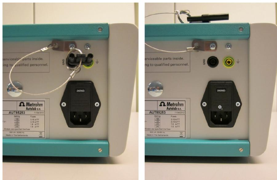
Figure 1077 The PGSTAT302F can be set to normal mode (left) or to floating mode (right) using the provided short-circuit plug
