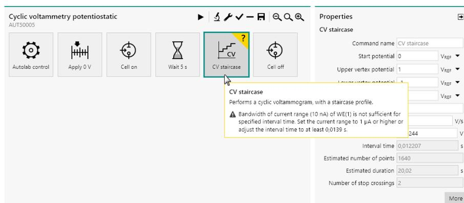
Figure 1064 Warnings are provided when bandwidth limitations are encountered
