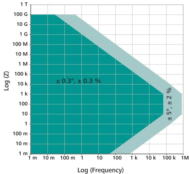
*Figure 1214* Contour map of the PGSTAT302N/FRA32M combination
