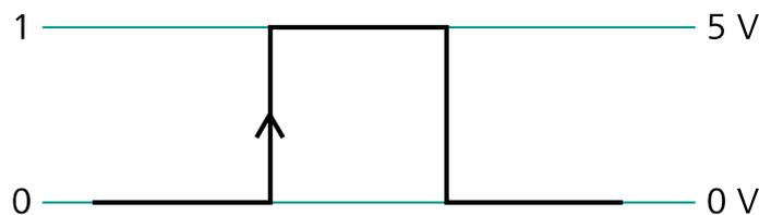
Figure 1124 Rising edge TTL trigger
