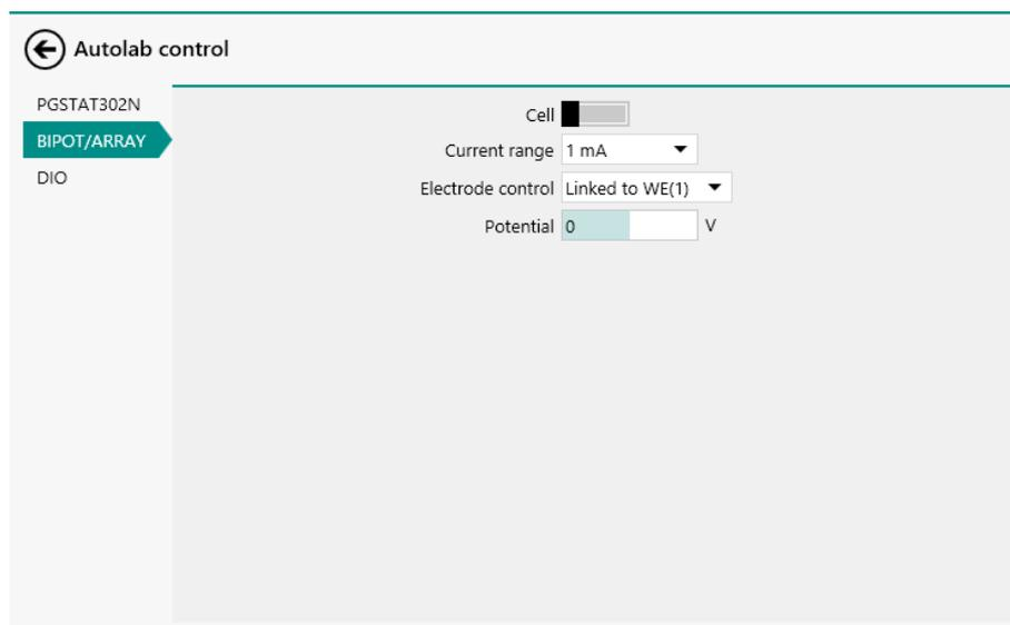
Figure 1151 The BIPOT/ARRAY module settings are defined in the Autolab control command
