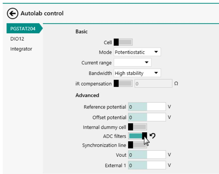
Figure 1115 The ADC filter property is provided in the Autolab control command
