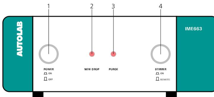
Figure 1224 Overview of the front panel of the IME663
