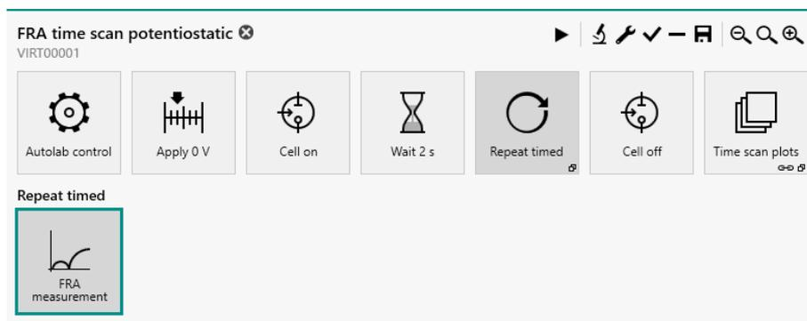
Figure 724 The default FRA time scan potentiostatic procedure
