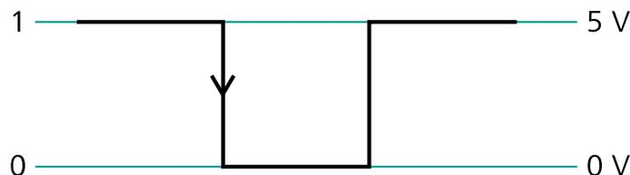
Figure 1125 Falling edge TTL trigger
