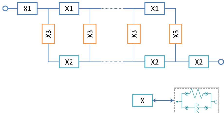
Figure 465 Overview of the general transmission line model used in the B2 element
