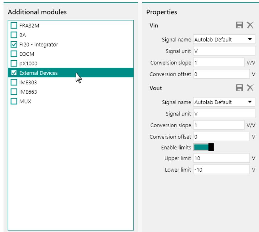
Figure 1111 The External Devices module adds the ADC164 or on-board ADC to the hardware setup
