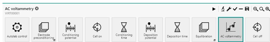
Figure 646 The default AC voltammetry procedure
