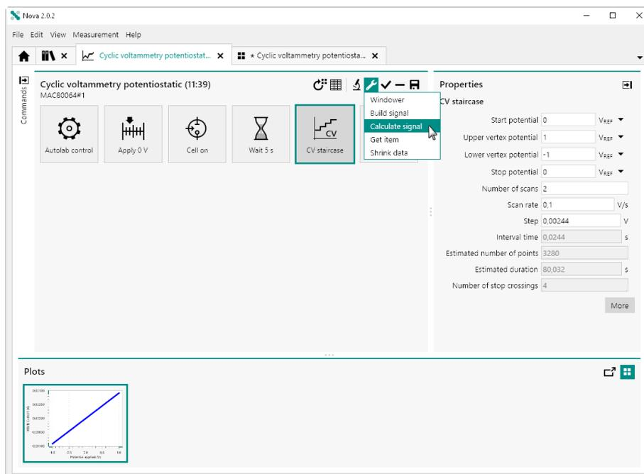
Figure 45 The data handling shortcut button can be used to add data handling commands easily
