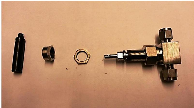
**Fig. 35 Needle valve parts from left: handle, adjustment nut, fastening nut, valve body**
