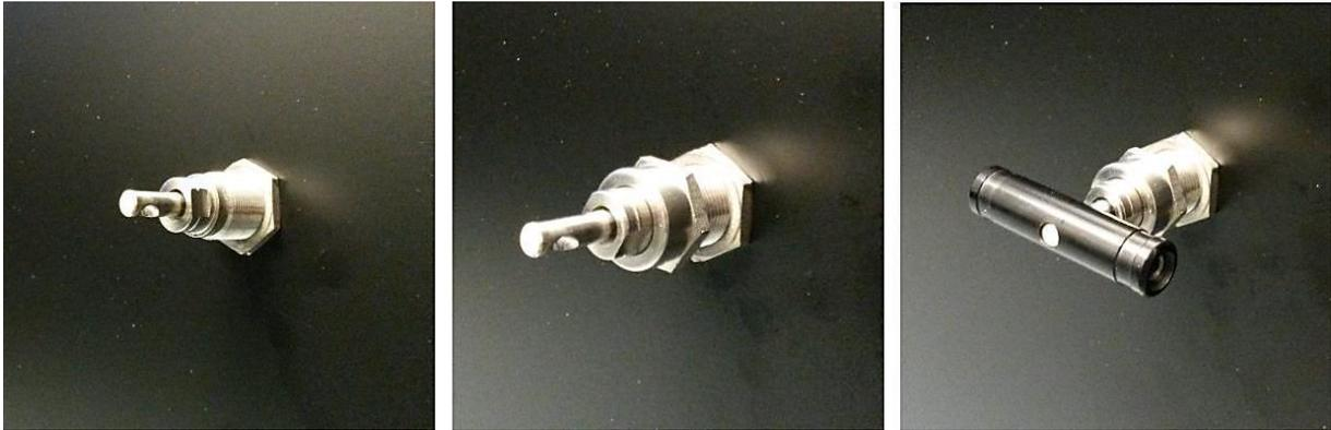
**Fig. 36 Steps for mounting a needle vale; fastening nut, adjustment nut and handle**
