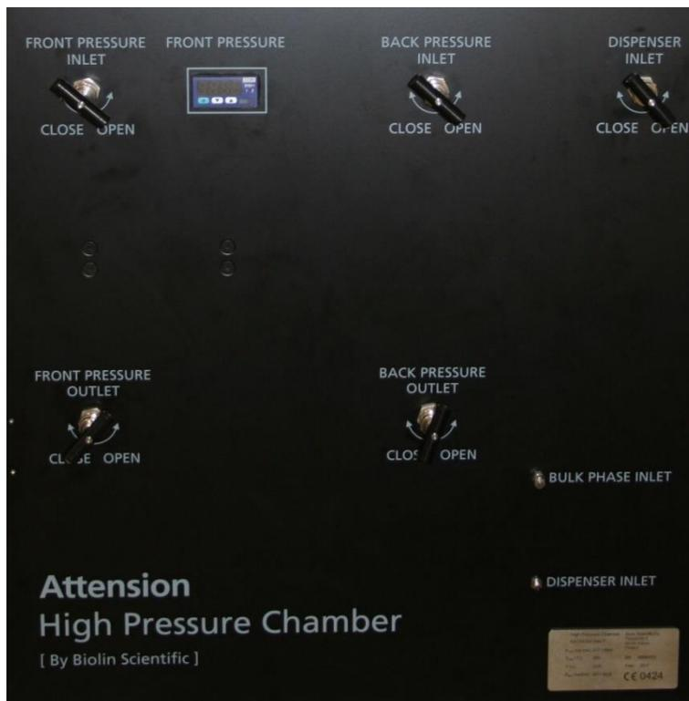
**Fig. 14 Valve panel on the safety cabinet door**
