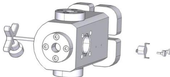
**Fig. 8 Mounting the thermal switch**
