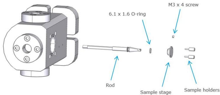
**Fig. 6 Mounting the sample stage**
