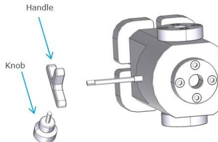
**Fig. 7 Mounting the knob and handle**
