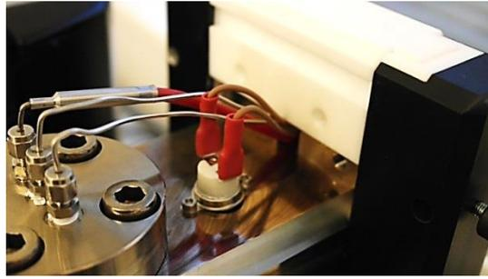
**Fig. 2 Over temperature switch is located on top of the chamber**
