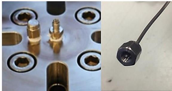
**Fig. 33 NPT male connector on the chamber and the cap at the end of the tube**
