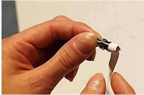
**Fig. 29 Making the Teflon seal**
