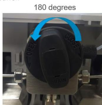
**Fig. 20 Drain valve knob**
