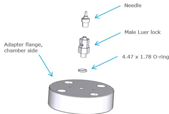
**Fig. 9 Mounting the needle**
