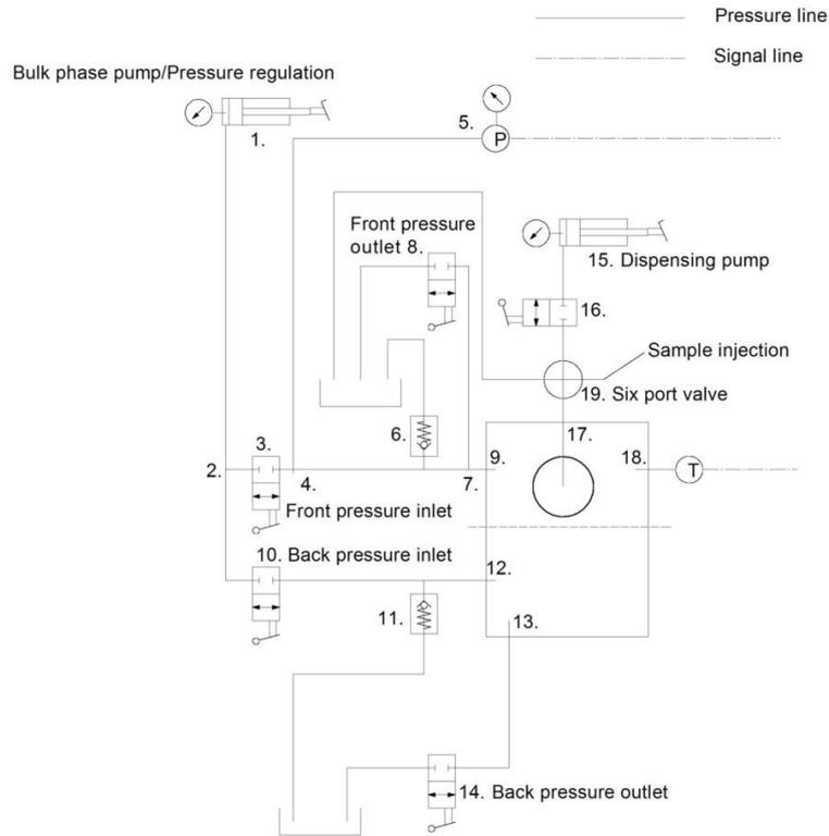
**Fig. 11 Schematics of the valves and fluid lines into high pressure chamber when two manual pumps are connected. Please note that pump symbols of the schematics will vary with different pump configurations, but the valve and fluid lines will remain the same.**
