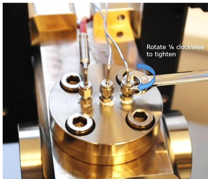
**Fig. 16 Closing the tube connection**
