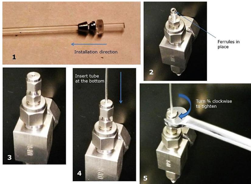
**Fig. 32 Connecting tube to a tube fitting: Ferrules (1), Ferrules inside tube fitting (2), tube fitting in valve opening (3), Tube inserted (4), tightening the cap nut (5).**
