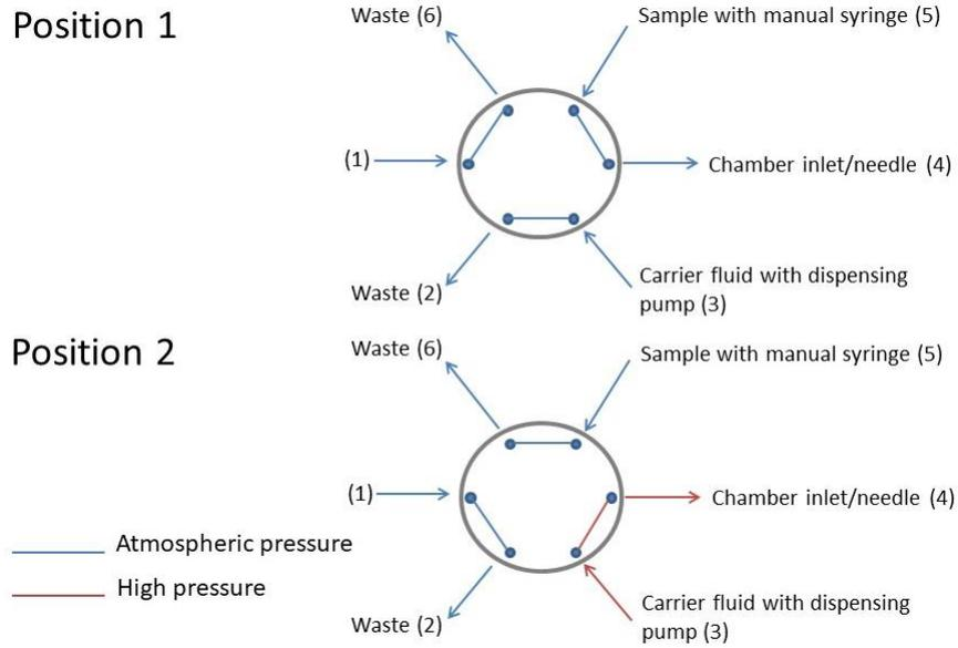
**Fig. 13 Six port valve connections.**
