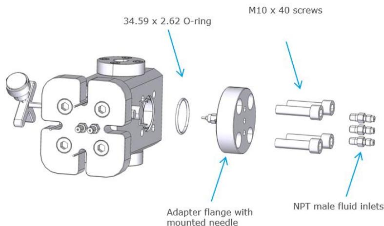
**Fig. 10 Adapter flange assembly**
