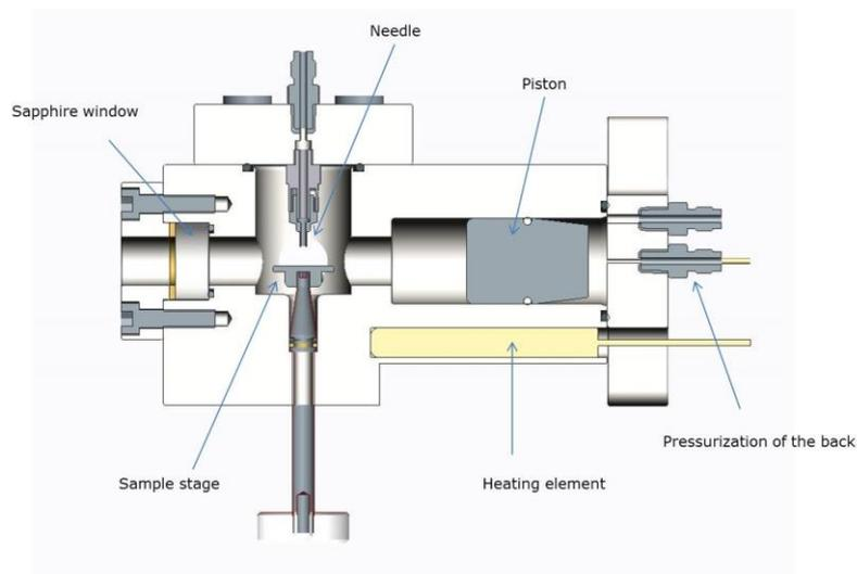
**Fig. 3 Schematic of the chamber**
