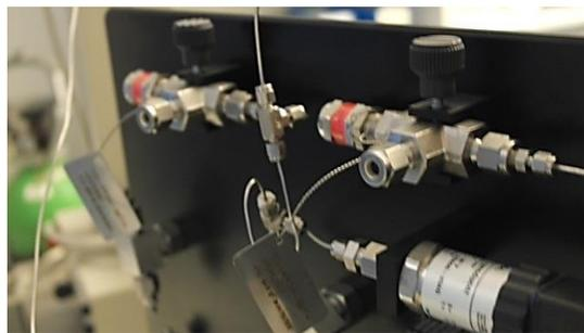
**Fig. 1 Over pressure valves for back and front parts of the chamber**
