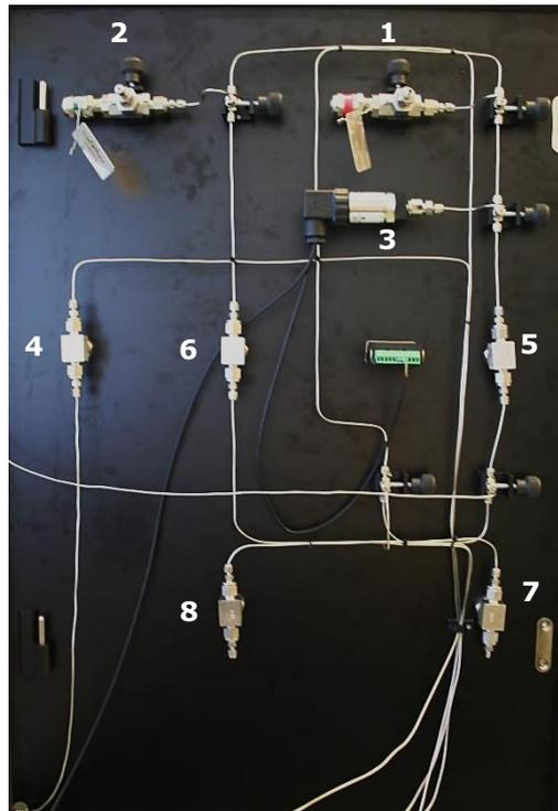
**Fig. 34 Back of the valve panel. The panel contains the over pressure valves for front (1) and back (2) of the chamber, pressure transducer (3), Sample inlet valve (4), Front side inlet valve (5), Back side inlet valve (8), Front side release valve (7) and Back side release valve (8).**
