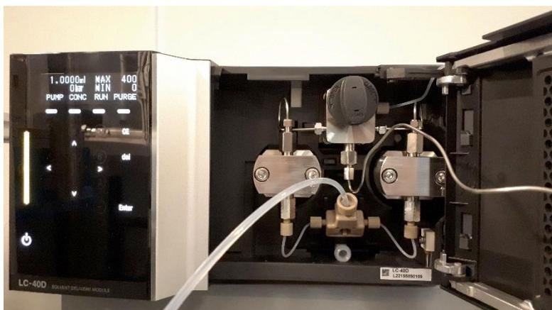
**Fig. 19 Automatic HPLC pump controller keypad and parts inside front cover**
