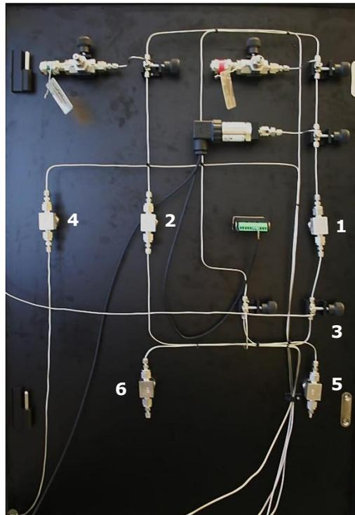
**Fig. 15 Connection at the back of the valve panel; connection to front part of the chamber (1), connection to back part of the chamber (2), Connection to the pump for pressurizing front and back parts (3), Connection to sample pump and needle (4), Connections to release bottle for both front (5) and back (6) parts of the chamber.**
