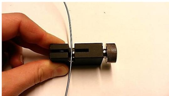
**Fig. 31 Using tube cutter tool**
