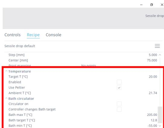
**Fig. 27 Peltier controls in the software**
