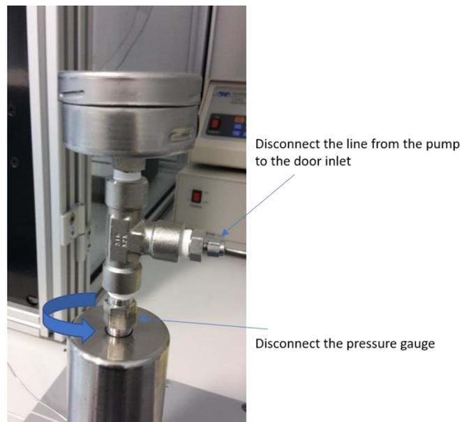
**Fig. 17 Disconnecting the pressure gauge**
