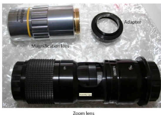
Magnification lens is attached to zoom lens with adapter.
