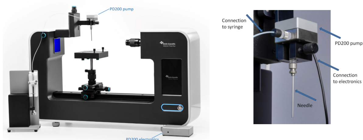
Theta Flow with PD200 and automated C201 dispenser.
