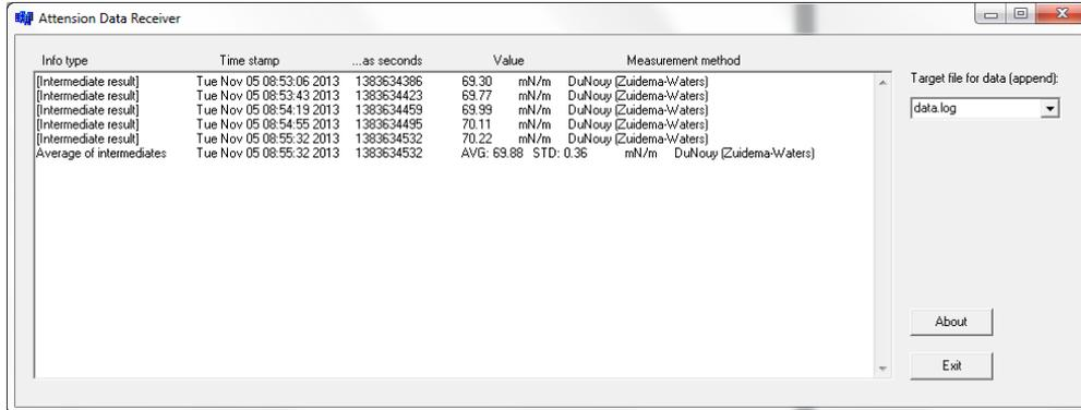
**Figure 8:** Attension Data Receiver to transfer measurement results to PC, including the intermediate results of a multi-round measurement.
