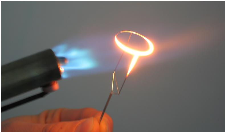
**Figure 7:** Cleaning a Du Noüy ring with a Bunsen burner.
