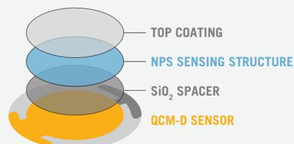
Acoulyte sensors are QCM-D sensors with a SiO<sub>2</sub> spacer layer deposited on the top gold electrode. The NPS structure is then deposited on top of this layer. The sensor surface can be covered by a top coating if desired.
