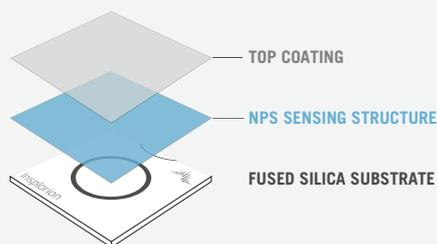
The dimensions of XNano and X1 sensors are 9.5x9.5x1 mm. The NPS sensing structure is deposited on a fused silica substrate. The sensor surface can be covered by a top coating if desired.
