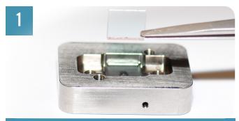
Mount the sensor chip in the titanium cartridge. If desired, the sensor chip can be precoated with the nanomaterial or thin film to be studied.
