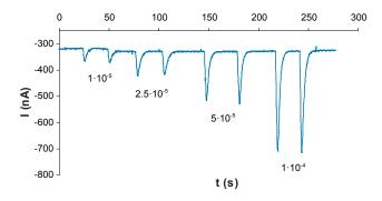
Analysis of hydrogen peroxide between  $1\cdot 10^{-5}~\text{M}$  and  $1\cdot 10^{-4}~\text{M}$  is presented in the figure.
