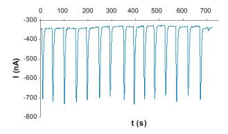
Amperometric detection of hydrogen peroxide in a flow injection analysis system with our easy to use Flow-cell. The amperometric responses for  $1\cdot 10^{-4}$  M  $H_2O_2$  at a ref. 710 electrode do not show any fouling effect. RSD% = 3.2, n = 15.
