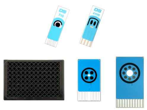
Disposable Screen-Printed Prussian Blue/Carbon Electrodes (refs. 710, X7710, 4W710, 8W710 and 96X710) are ideal for the determination of hydrogen peroxide at a low detection potential. These electrodes are recommended for the development of enzymatic biosensors based on oxidases, for working with microvolumes and for decentralized assays.
