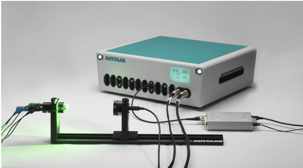
Figure 1 – The Optical Bench, including the LED driver, optical rail, light source and photodiode holder
