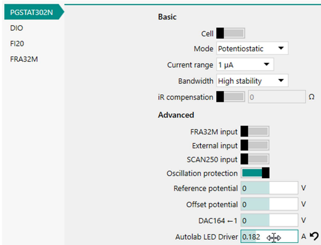
Figure 30 – Adjusting the driving current using the slider provided in the Autolab control dialog
