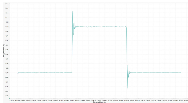
Figure 5. A positive feedback measurement of the circuit from Figure 1, dummy cell (c), with an acceptable iR compensation value of 95 Ω.
