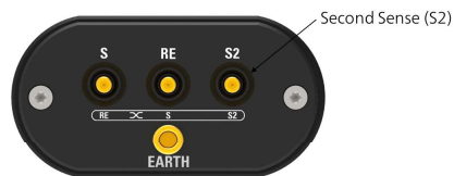
Figure 35 Second Sense (S2) connection on the Buffer box of the Pure signal bridge
