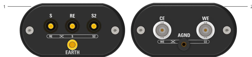
Figure 61 Connectors and labeling on the Pure signal bridge (Buffer (1) and Splitter (2) boxes).
