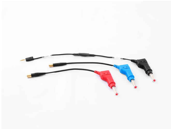
Figure 32 Adaptive cables used for high frequency measurements
