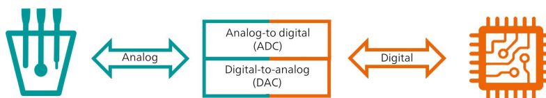
Figure 18 Basic representation of the signal path from the electrochemical cell (left) to the digital electronics of the instrumentation (right). Analog path - green, Digital path - orange.
