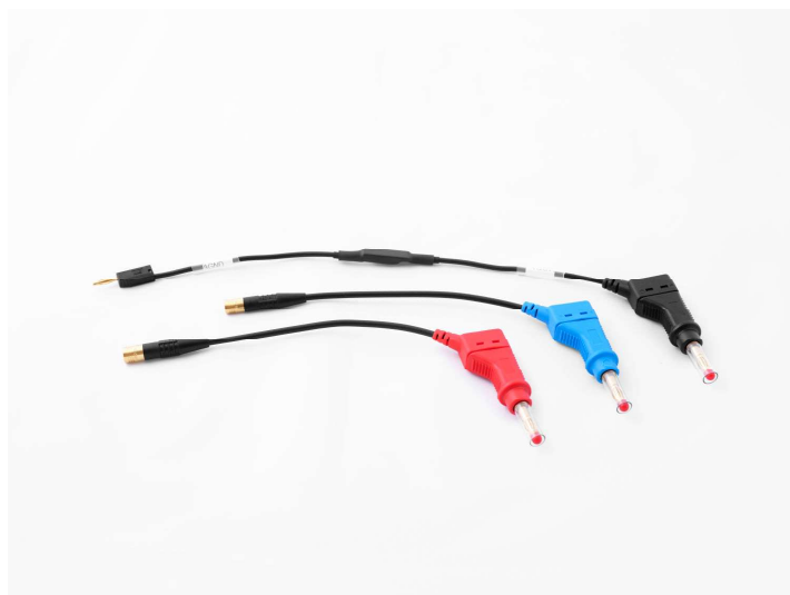
Figure 9 High frequency (HF) cables used for EIS measurements at frequencies higher than 1 MHz, 0.25 m with 4 mm banana connectors.
