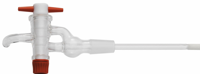
Figure 8 Gas inlet with frit and PTFE stopcock
