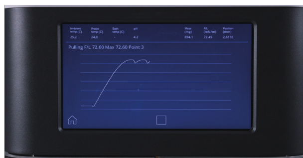
Live measurement view during surface tension measurement with a Du Noüy ring
